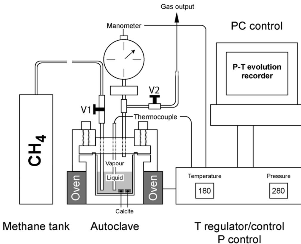
Figure 4.9. Experimental device; calcite fragments are located in the liquid water phase inside a gas sampling autoclave. The autoclave is pressurized from a methane tank, by opening the valve 1 (*V*<sub>1</sub>) through an injection tube. Valve 2 allows gas to exit causing a drop of pressure.
