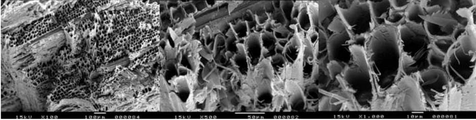
Fig. 3.9a-c Untreated simaruba, fracture surface after bending test
