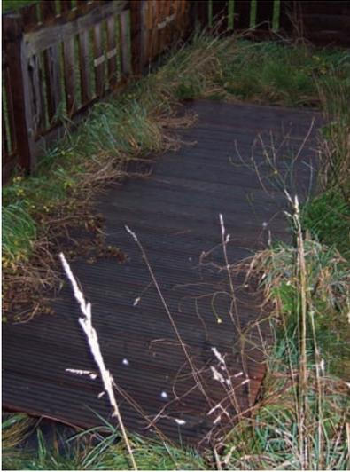
**Fig. 10.2** Three-year outdoor exposure of heat-treated Norway spruce terrace planking boards (2004-2006)
