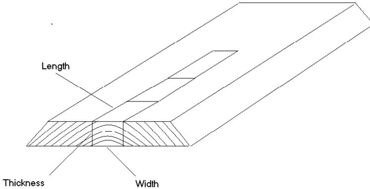
Fig. 11.1 Schematic overview of specimen preparation
