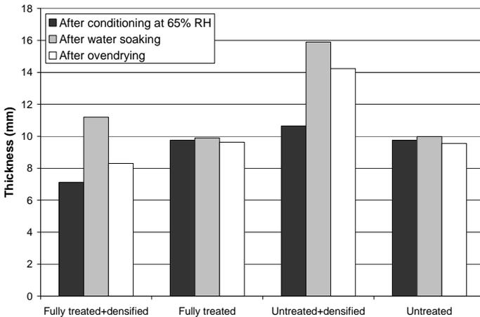
**Fig. 11.2** Thickness (radial direction) of treated and untreated radiata pine specimens after conditioning at 65% relative humidity (20°C), after water soaking (20°C), and after oven drying (102°C, 24 hrs)
