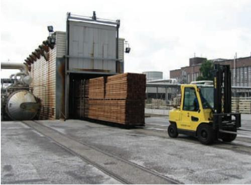
Fig. 1.4 Industrial kiln for the curing stage
