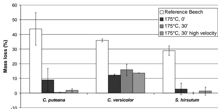
**Fig. 6.3b** Effect of different hydro-thermolysis process conditions on the mass loss of heat-treated birch after exposure to *C. puteana*, *C. versicolor* and *S. hirsutum* (CEN/TS 15083-1). High velocity: heating 2.75 K/minute; cooling down 2.0 K/minute.
