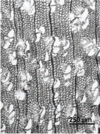
Fig. 3.4a First steam hydro-thermolysis trials on birch (cross section), radial cracks and collaps of the vessels
