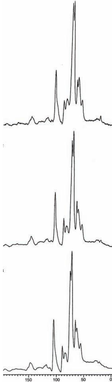
**Fig. 4.2** Standard CP-MAS <sup>13</sup>C-NMR spectra of untreated (top), intermediate (middle) and fully treated (below) Scots pinewood
