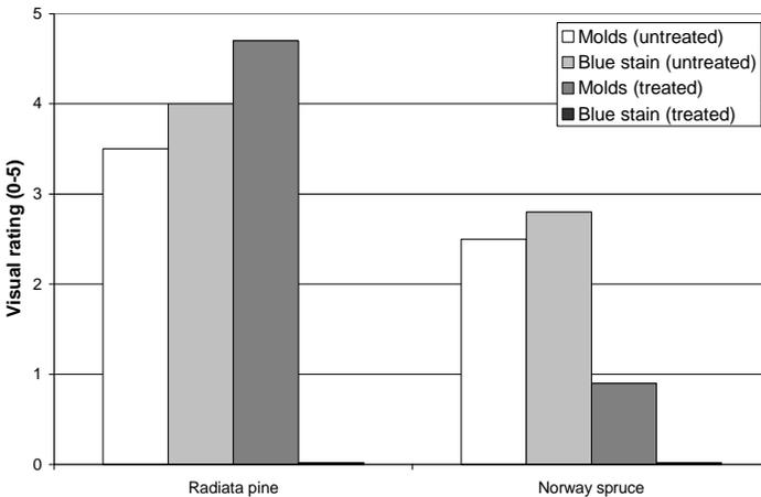
**Fig. 6.7** Visual assessment treated and untreated radiata pine and Norway spruce after 3 months exposure to molds and blue stain fungi according a modified EN 152 test. 0 = no fungal growth on the surface; 5 = severe fungal growth on the surface
