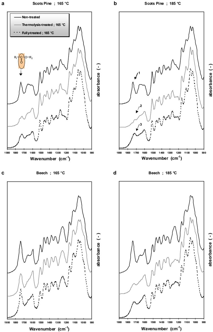
**Fig. 2a–d** FTIR spectra of heat treated Scots Pine and beech. Untreated, half-treated and fully treated wood, low temperature (a and c) and high temperature (b and d) treatment in the hydrothermal stage of the process
