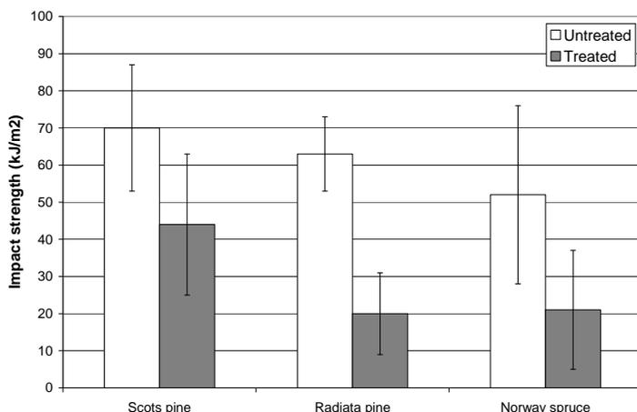
**Fig. 9.1** Impact strength of untreated and heat-treated Scots pine, radiata pine and Norway spruce defect free specimens. Treatment conditions: hydro-thermolysis 165°C, 30 minutes; curing 180°C, 6 hrs
