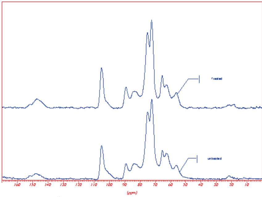
**Fig. 8.3** CP MAS <sup>13</sup>C NMR spectra after fungal exposure in ground contact (EN 252) of untreated (below) and heat-treated (above) Norway spruce
