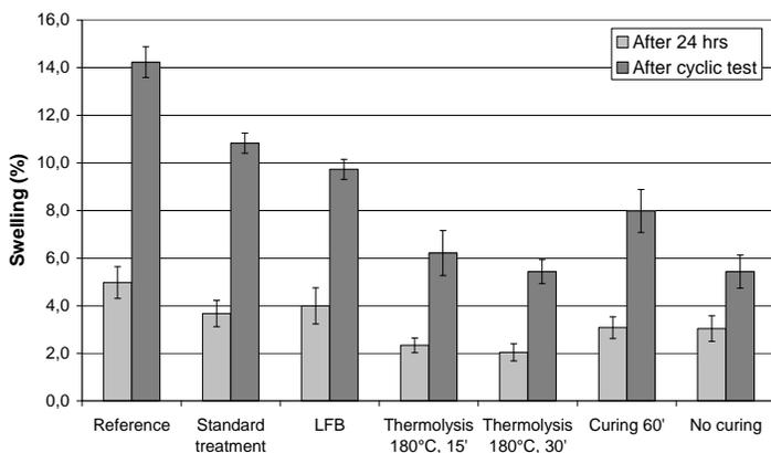
**Fig. 13.5** Swelling of treated and untreated particleboard test samples (MUF, 13.5%) after 24 hours immersion in water at 20°C and after the cyclic test. Standard treatment: steam hydro-thermolysis 165°C, 30 min; curing 180°C, 30 min
