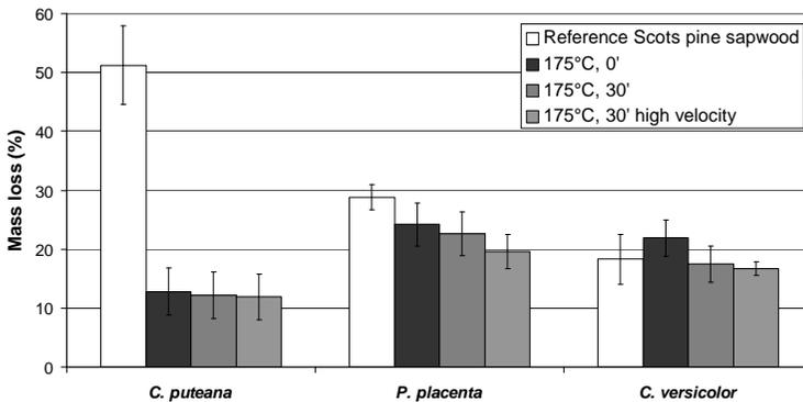
**Fig. 6.3a** Effect of different hydro-thermolysis process conditions on the mass loss of heat-treated radiata pine after exposure to *C. puteana*, *P. placenta* and *C. versicolor* (CEN/TS 15083-1). High velocity: heating 2.75 K/minute; cooling down 2.0 K/minute.
