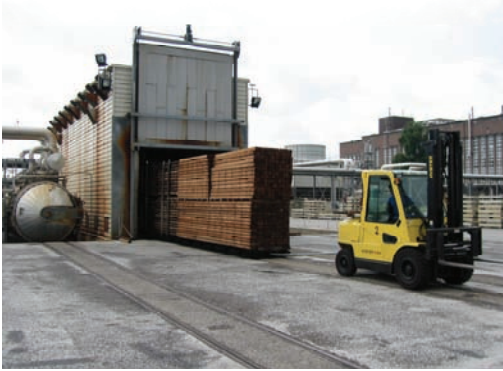
Fig. 1.4 Industrial kiln for the curing stage
