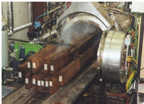
**Fig. 1.1** Pilot plant for the hydro-thermolysis stage
