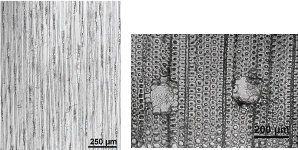
**Fig. 2.5a,b** Liquid full hydro-thermolysed treated Scots pine (tangential and cross section), damaged parenchyma ray cells (a) and epithelial cells of resin canals (b). The ray tracheids are still intact
