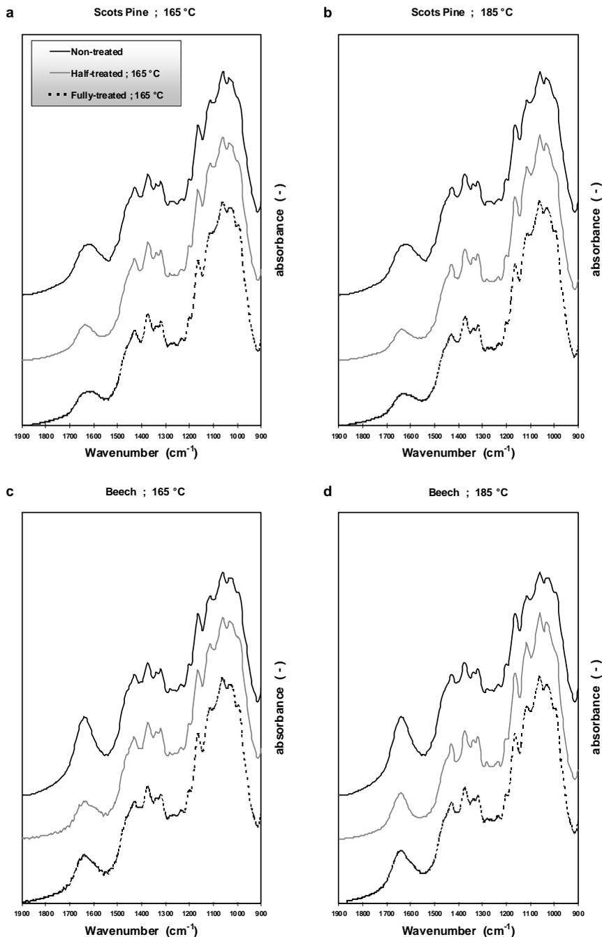
**Fig. 5a–d** FTIR spectra of  $\alpha$ -cellulose isolated from heat treated Scots Pine and beech. Untreated, intermediate and fully treated wood, low temperature (a and c) and high temperature (b and d) treatment in the hydrothermal stage of the process
