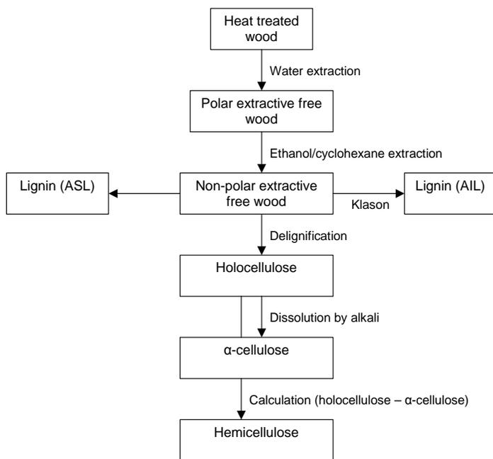
**Fig. 5.1** Wet chemical analysis procedure of untreated, intermediate and heat-treated Scots pine
