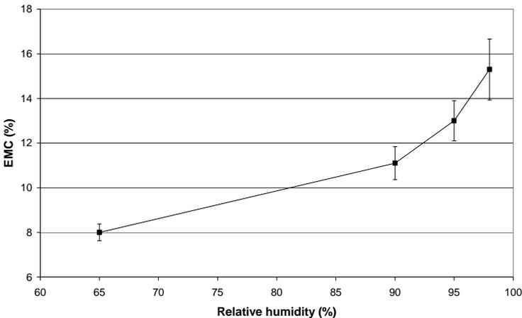
**Fig. 10.7** Equilibrium moisture content (EMC) of heat-treated Norway spruce terrace planking boards (cross section 27x125 mm) at 65%, 90%, 95% and 98% relative humidity (20°C) after three years outdoor exposure
