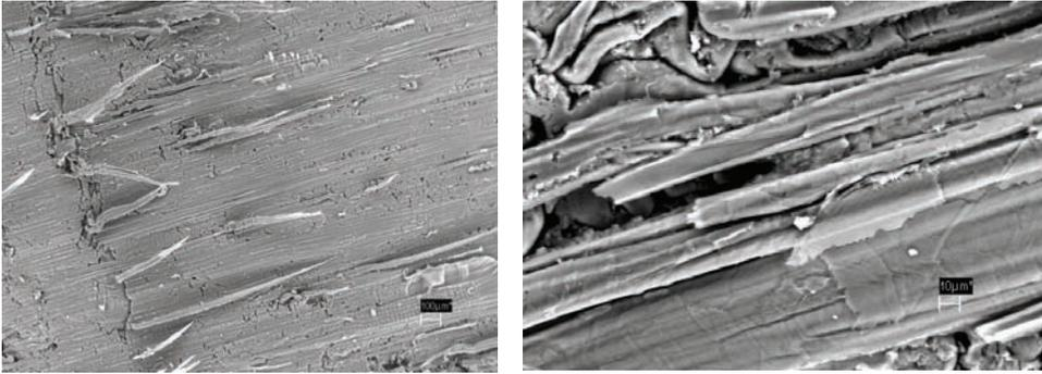
**Fig. 12.2** (a) Scanning electron micrographs of heat-treated poplar wood just after the first hydrothermolysis treatment step showing apparently rigidified wood cells that have not detached from the wood surface, that have not entangled and where there is none or very little of the molten matrix intercellular material usual in welded timber (Gfeller et al. 2003). (b) Higher magnification detail of (a)
