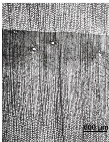
**Fig. 2.2b** Liquid full hydro-thermolysed treated Norway spruce (cross section), with larger annual rings and a gradual transition from earlywood to latewood. No tangential cracks in the latewood section are visible
