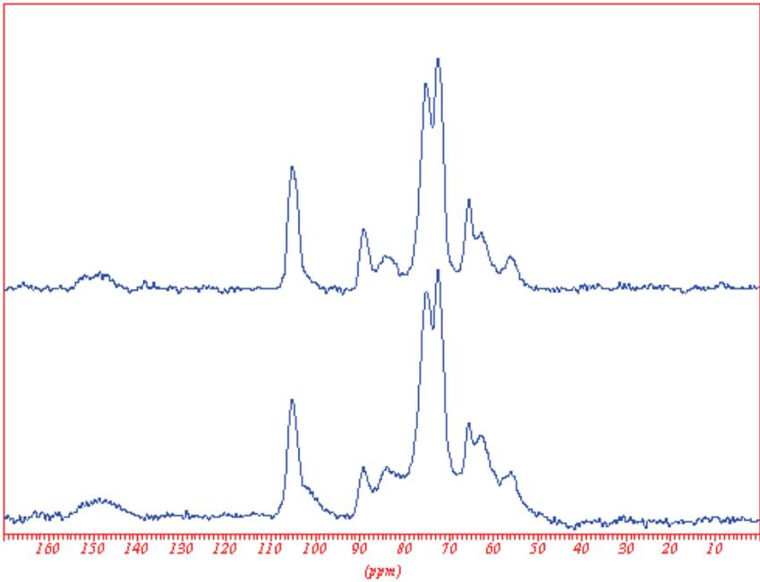
**Fig. 8.2** CP MAS <sup>13</sup>C NMR spectra after fungal exposure in ground contact (EN 252) of untreated (below) and heat-treated (above) radiata pine
