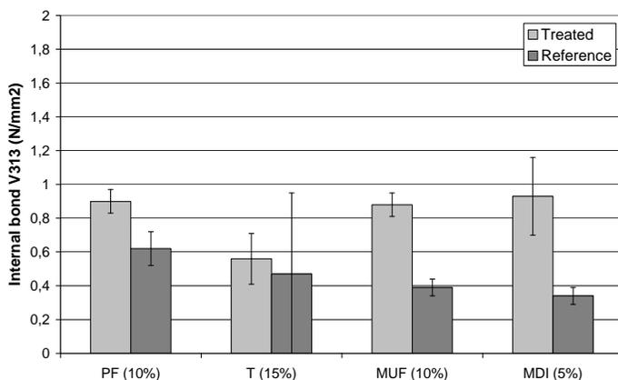
**Fig. 13.12** The internal bond of treated and untreated particleboard test samples after the cyclic test (V313). The effect of different adhesives. Hydro-thermolysis: LF 185°C; curing: 180°C, 240 min
