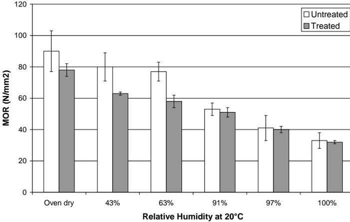
**Fig. 9.4a** Effects of conditioning on the bending strength of heat-treated and untreated radiata pine specimens (defect free). Treatment conditions: hydro-thermolysis 165°C, 30 minutes; curing 180°C, 6 hrs
