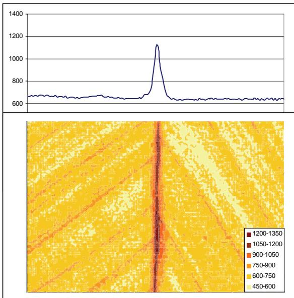
**Fig. 12.4** X-ray microdensitometry map of friction welded birch wood after final dry heat cure treatment. Upper microdensitometry graph expresses density in kg/m<sup>3</sup> of the wood as a function of the sample weld interface position in mm. The bottom panel is the colour intensity microdensitometry map expressing increasing density in kg/m<sup>3</sup> by progressive darkening. Scale of sample weld interface position is the same for the two panels
