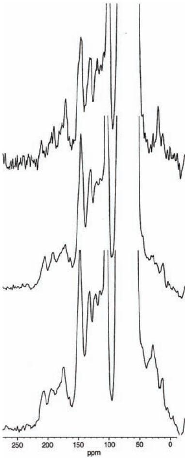
**Fig. 4.1** Expanded to maximize 100-200 ppm region CP-MAS <sup>13</sup>C-NMR spectra of untreated (top), intermediate (middle) and fully treated (below) Scots pinewood
