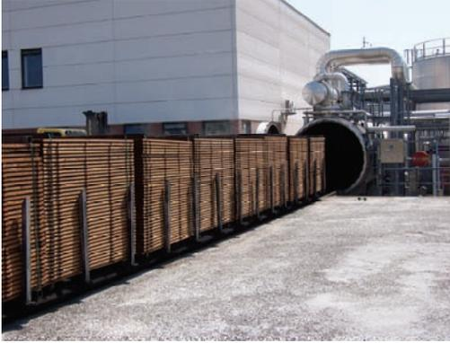
**Fig. 1.2** Industrial plant for the hydro-thermolysis stage
