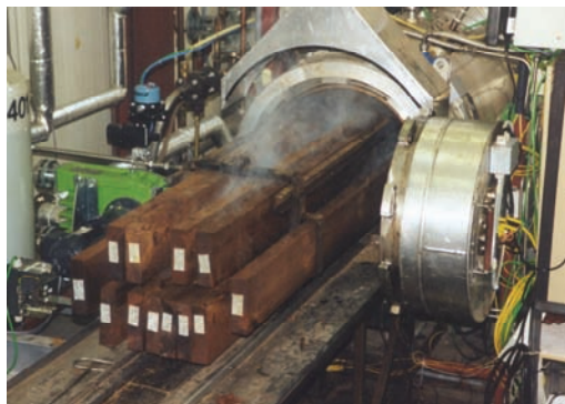
Fig. 1.1 Pilot plant for the hydro-thermolysis stage
