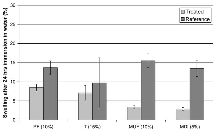
**Fig. 13.8** Swelling of treated and untreated particleboard test samples after 24 hours immersion in water at 20°C. The effect of different adhesives. Hydro-thermolysis: LF 185°C; curing: 180°C, 240 min
