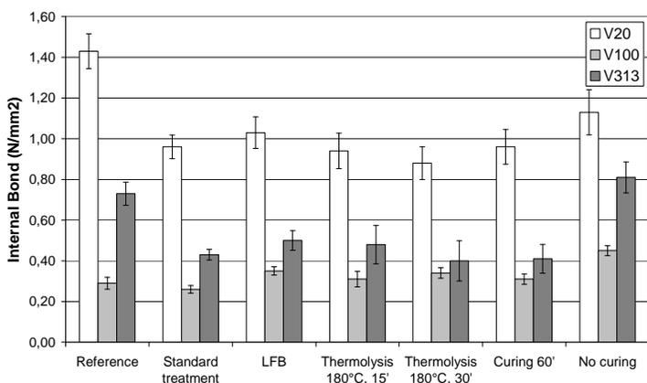
**Fig. 13.6** Internal bond of treated and untreated particleboard test samples (MUF, 13.5%) at 20°C (V20), after the boiling test (V100) and after the cyclic test (V313). Standard treatment: steam hydrothermolysis 165°C, 30 min; curing 180°C, 30 min
