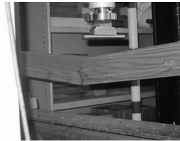
Fig. 2.7b The typical fracture of a completely treated Norway spruce specimen after a bending test
