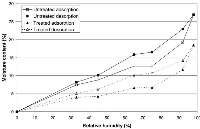
**Fig. 9.5** Moisture content of untreated and heat-treated radiata pine conditioned at different relative humidity (hysteresis). Treatment conditions: hydro-thermolysis 165°C, 30 minutes; curing 180°C, 6 hrs
