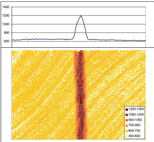
**Fig. 12.3** X-ray microdensitometry map of friction welded hydrothermally treated birch wood. Upper microdensitometry graph expresses density in kg/m<sup>3</sup> of the wood as a function of the sample weld interface position in mm. The bottom panel is the colour intensity microdensitometry map expressing increasing density in kg/m<sup>3</sup> by progressive darkening. Scale of sample weld interface position is the same for the two panels
