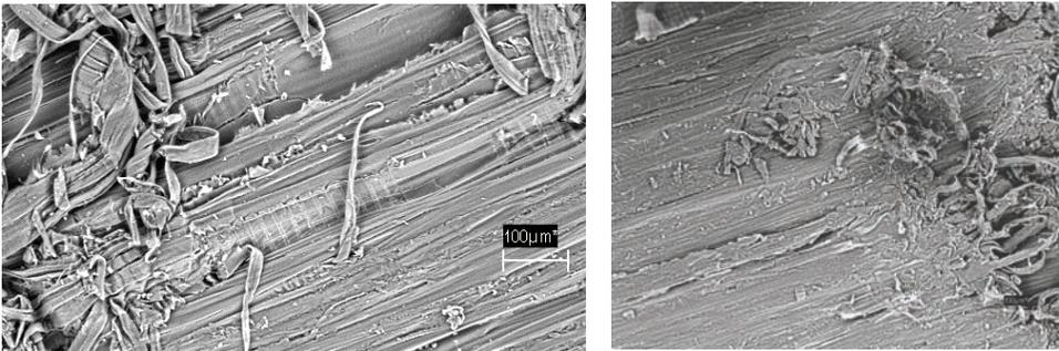
**Fig. 12.1** (a) Scanning electron micrograph of heat-treated poplar wood after the last dry heat curing step showing entangled cells where there is none or very little of the molten matrix intercellular material usual in welded timber. (b) Scanning electron micrograph of heat-treated birch wood just after the first hydro-thermolysis treatment step showing entangled cells where there is none or very little of the molten matrix intercellular material usual in welded timber
