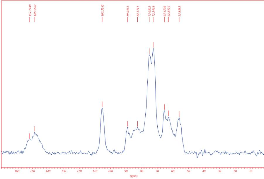
**Fig. 7.1a** CP-MAS <sup>13</sup>C-NMR spectra after *C. puteana* exposure (EN 113) of untreated Scots pine sapwood (mass loss 45.4%)
