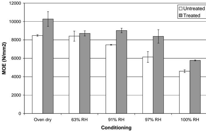
**Fig. 9.4b** Effects of conditioning on the Modulus of Elasticity of heat-treated and untreated radiata pine specimens (defect free). Treatment conditions: hydro-thermolysis 165°C, 30 minutes; curing 180°C, 6 hrs
