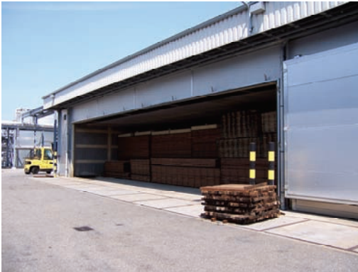
Fig. 1.3 Industrial kiln for pre-drying, drying and conditioning of timber during heat treatment
