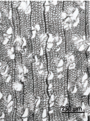
Fig. 3.4a First steam hydro-thermolysis trials on birch (cross section), radial cracks and collapses of the vessels
