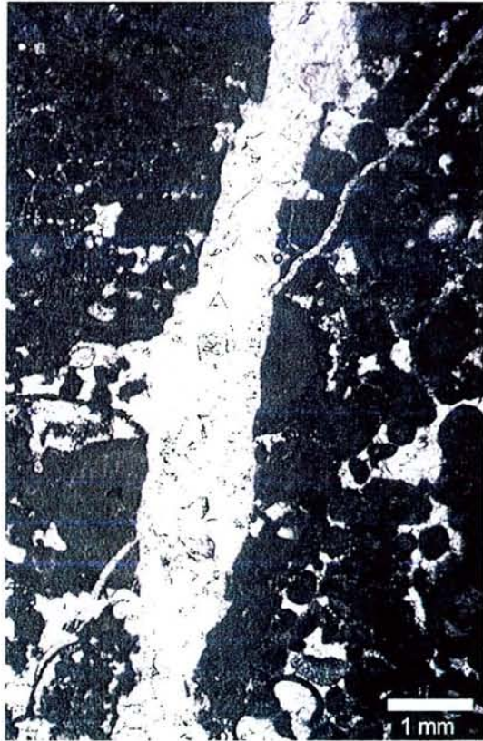
Fig. 7.4. A: small vertical fissure filled by calcite crosscutting thin subhorizontal stylolites from middle Oxfordian limestones in borehole HTM102 (2540: 218m). B: fissures (N30 strike) from N11 site (Bathonian-Bajocian limestones) filled by calcite. C-D: microphotographs thin calcite fissures crosscutting: C: mudstone (HTM102-2523: 111m) and D: oolitic limestones (HTM102-2536: 196m) cemented by pervasive calcite similar to that one of the thickest fissure (HTM102-2536: 196m).
