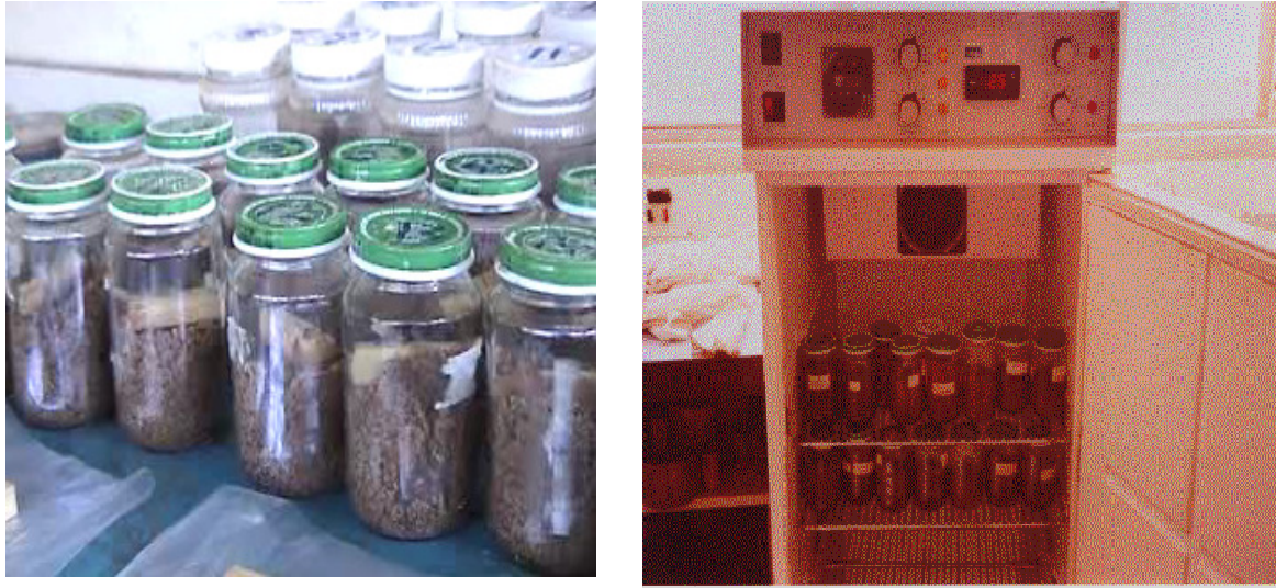
Figure 19. Termite test in the laboratory
