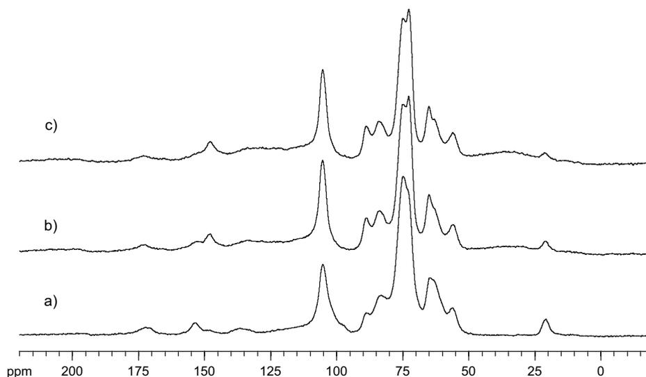
Fig. 2. CP/MAS <sup>13</sup>C NMR spectra of thermally modified or not beech sawdust: (a) unmodified sawdust; (b) heat treated at 240 °C during 5 h 30 min, WL = 17.7%; (c) heat treated at 240 °C during 21 h, WL = 23.6%.
