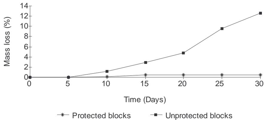
Figure 10: Mass loss measurements for control and propiconazole protected blocks exposed to *C. versicolor*
