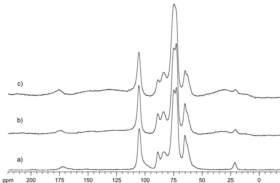
Fig. 3. CP/MAS  $^{13}\text{C}$  NMR spectra of thermally modified or not beech holocellulose fraction: (a) unmodified holocellulose fraction; (b) heat treated at  $240\text{ }^{\circ}\text{C}$  during 5 h 30 min, WL = 37%; (c) heat treated at  $240\text{ }^{\circ}\text{C}$  during 21 h, WL = 41%.
