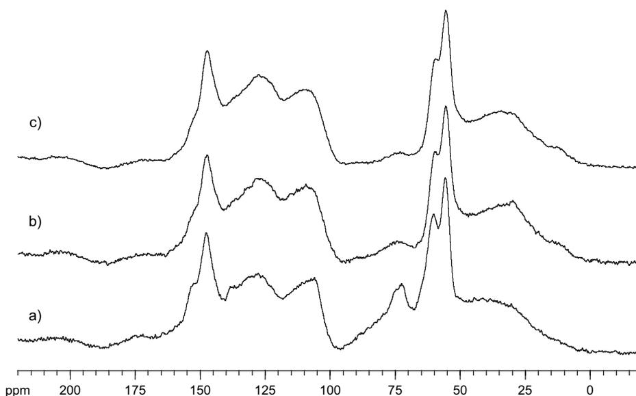
Fig. 4. CP/MAS  $^{13}\text{C}$  NMR spectra of thermally modified or not beech lignin fraction: (a) unmodified lignin fraction; (b) heat treated at  $240\text{ }^{\circ}\text{C}$  during 5 h, WL = 16.9%; (c) heat treated at  $240\text{ }^{\circ}\text{C}$  during 21 h, WL = 17.7%.
