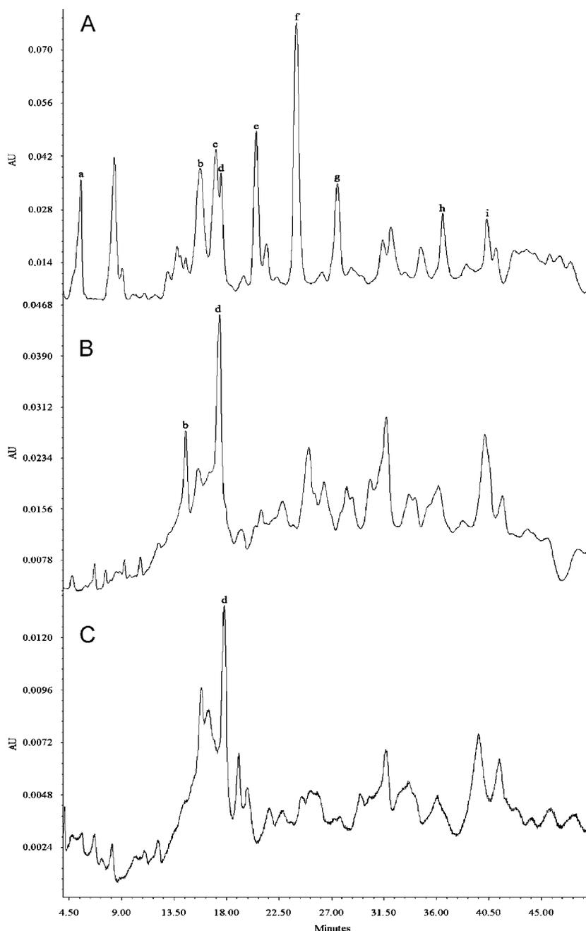
Fig. 1. Acetonetic extractives chromatograms at 280nm of wood beech dried at 103 °C (A), undried (B) and dried at 55 °C (C) Peak identities: a = protocatechuic acid, b = 2,6-dimethoxybenzoquinone, c = vanillic acid, d = catechin, e = vanillin, f = syringic acid, g = 3,5-dimethoxy-4-hydroxybenzaldehyde, h = coniferaldehyde, i = synapic acid.
