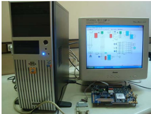
Figure III-15. Prototypage "FPGA in the Loop".
