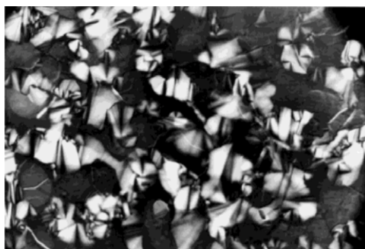
Figure IV-3. Characteristic texture of the hexagonal liquid crystal.
