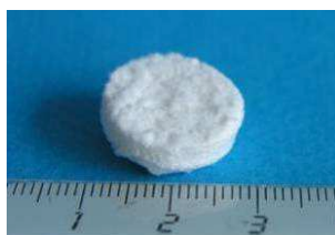
Figure IV-20 Photograph of a monolith prepared at 7% PFOBr; R=3 , pH=0.025 .
