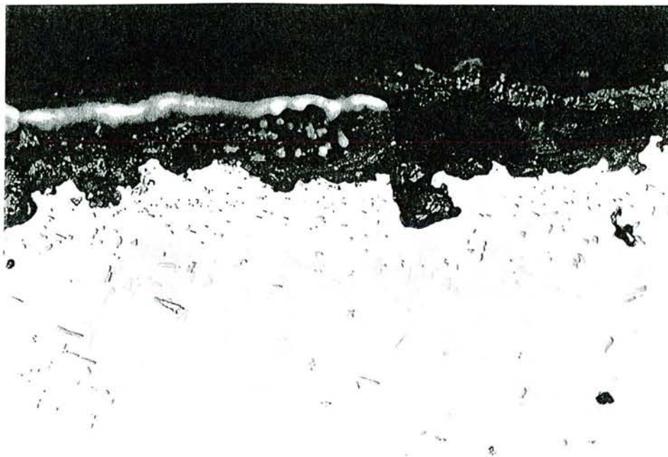
Figure VI-26 : SRR 99 – Pd/Ni HA lot 2 – Oxydation de 1005 cycles (x 437).
