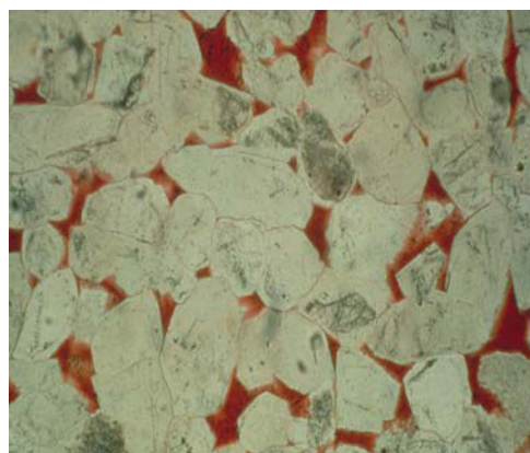
d. Thin section of epoxy pore cast Fontainebleau sandstone.
