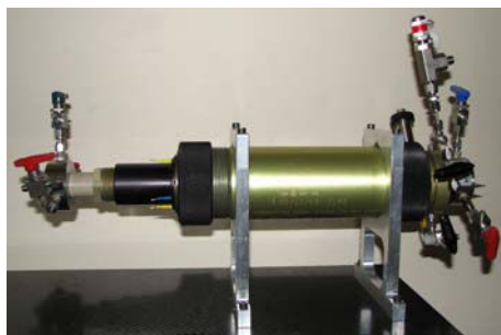
a. The X-ray core-holder used for CT imaging during our experiments.
