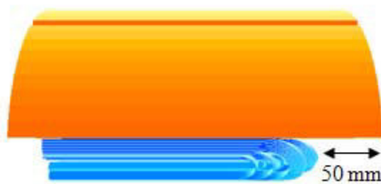
Figure 107 – Iron yoke coil in the final configuration: the yoke is 50 mm longer than the coil.
