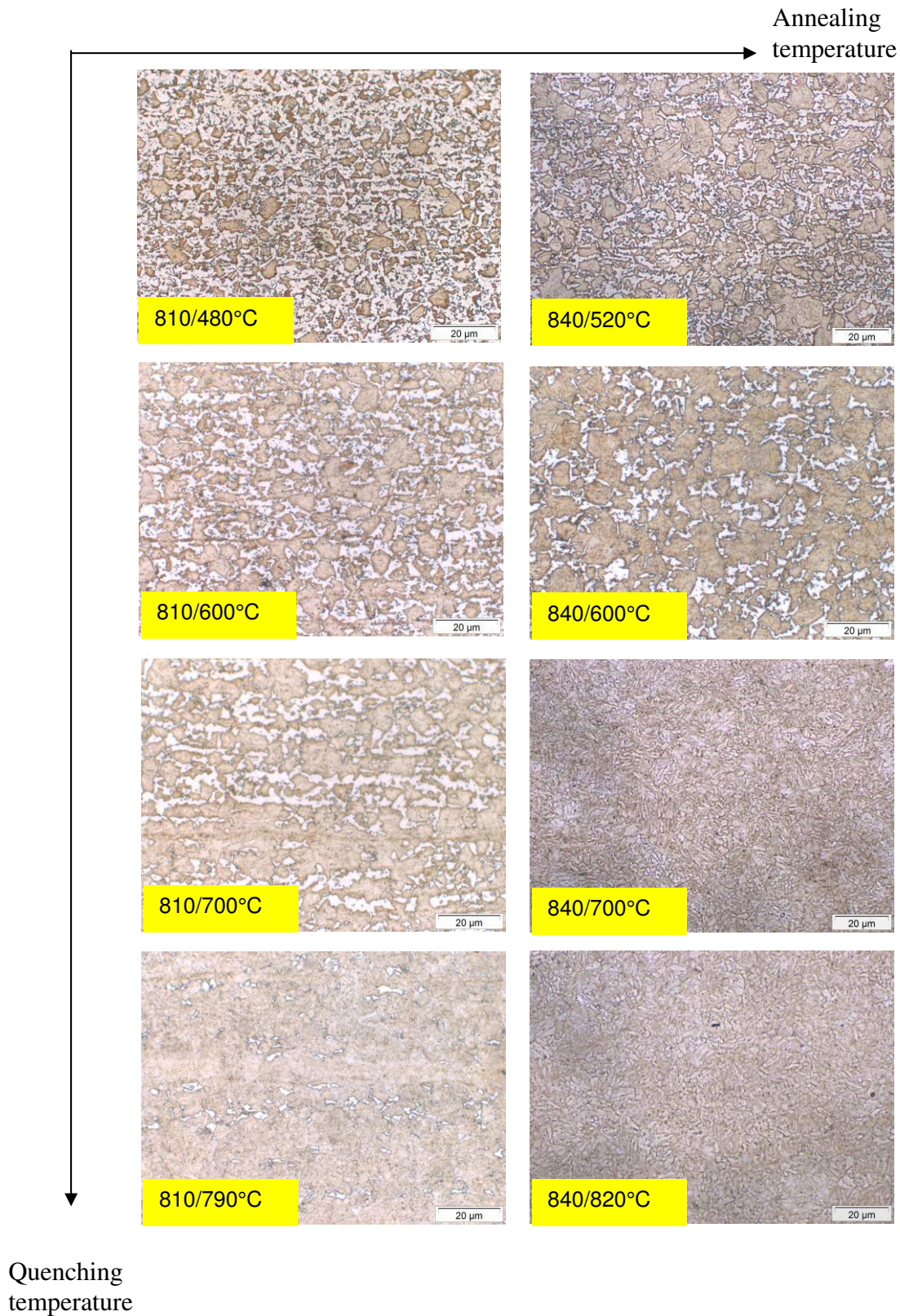
Figure II.11. Microstructure evolution with annealing/quenching temperature. Picral and metabisulfite etching. White-etching phase is ferrite, dark-etching phase is martensite.
