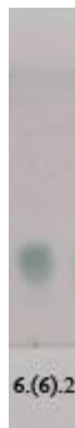
Figure 20 Silica gel thin layer chromatography of the purified fractions F6.(6).2 eluting from third silica gel column chromatography. Mobile phase; hexane:ethyl acetate, 1/1(v/v), detection with \rho -anisaldehyde spray.
