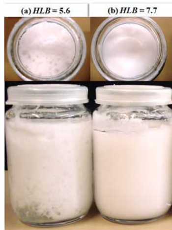
Figure 10: Highly concentrated emulsions prepared with 2 wt. % NaCl and f_w = 0.95 . a) HLB = 5.6 (less stable) b) HLB = 7.7 (more stable)
