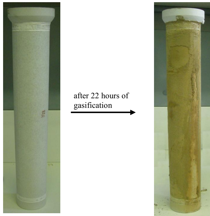
Figure 20: Catalytic ceramic candle before and after the whole gasification test of 22 hours
