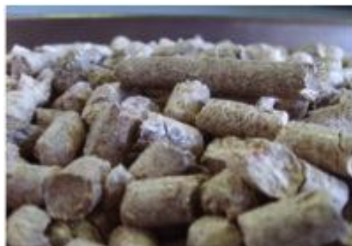
Figure 9: MXG pellet (6 mm of diameter)
