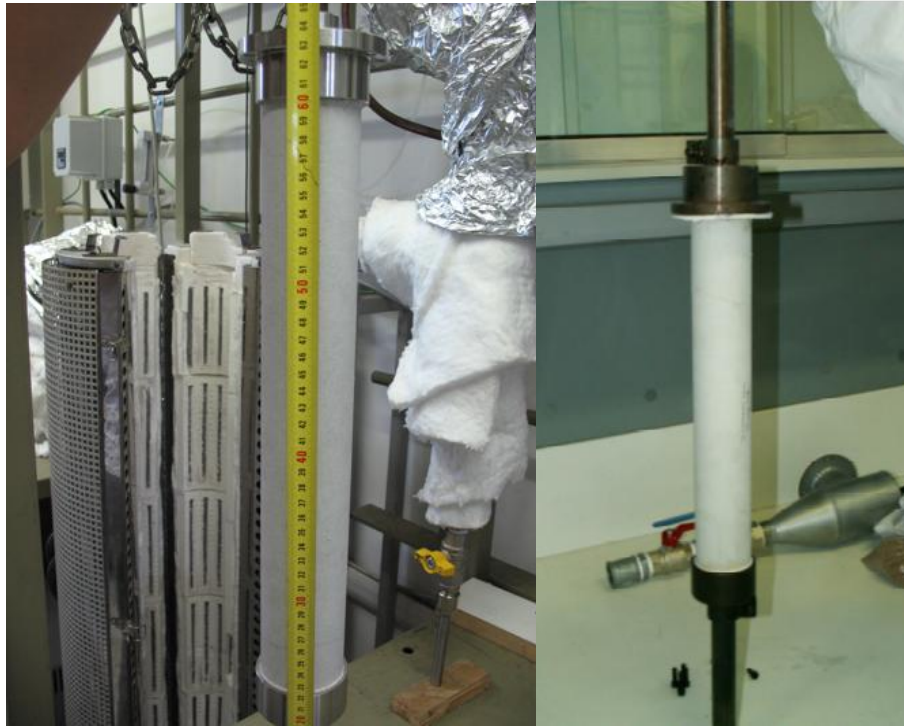
Figure 4: Pictures of the catalytic/non catalytic filter candle showing the dimension and the blockage system in the reactor A- freeboard.
