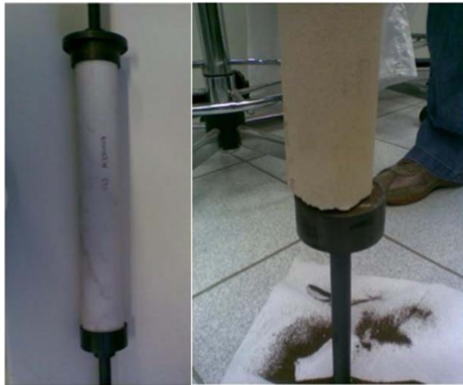
Figure 14: The main problem experienced in our experiments was the breakage of the ceramic candle (picture on the right)
