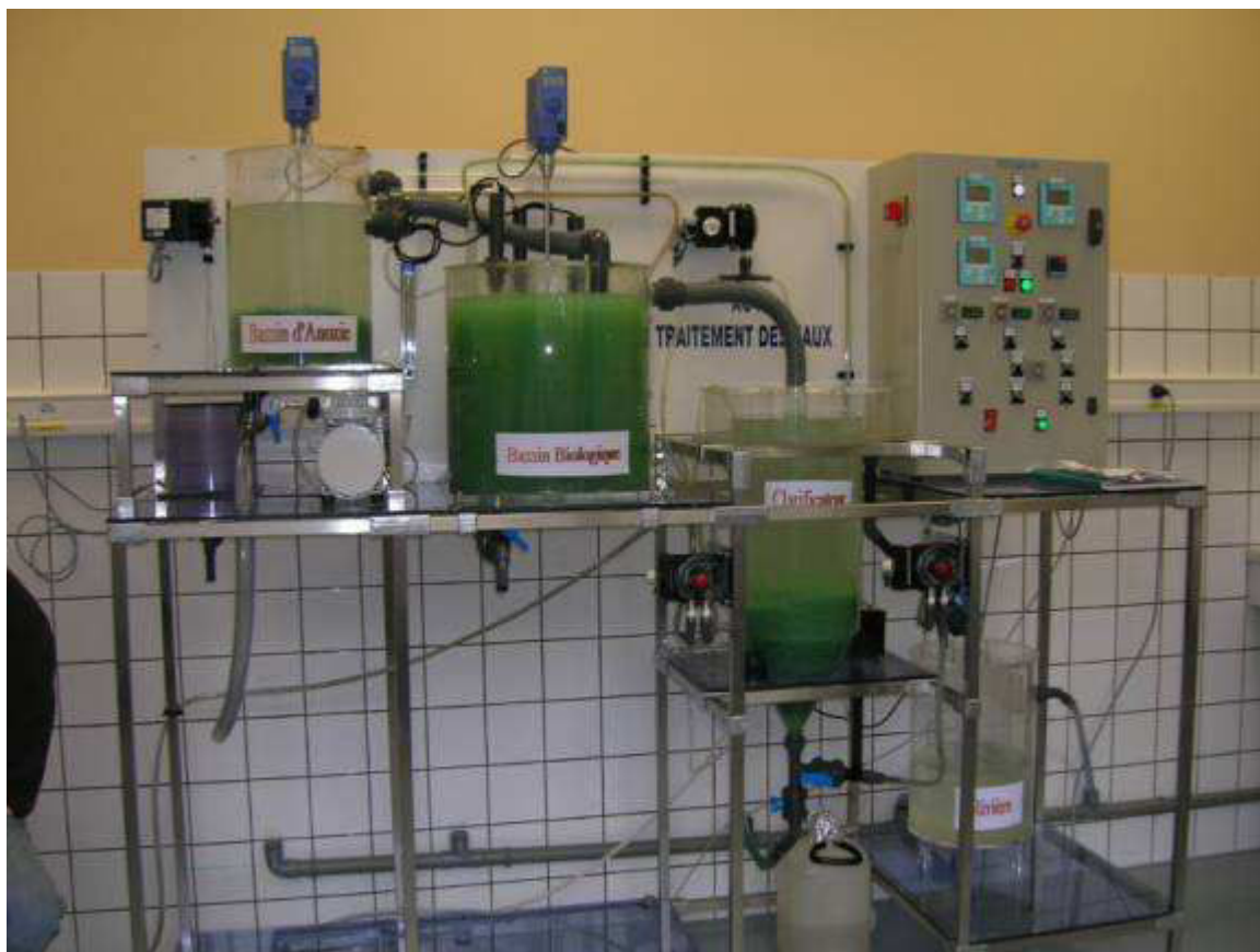
Figure 1. Lab scale pilot used for the fungal treatment of wastewater from the paper mill
