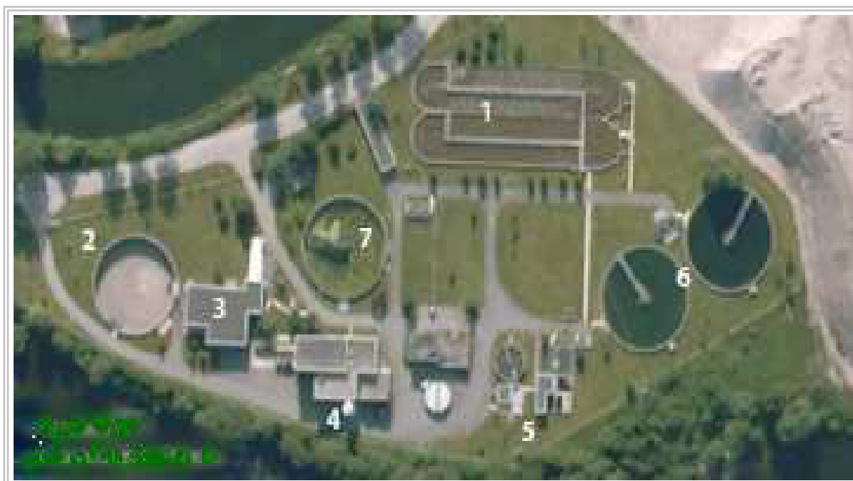
Figure II.1. Plan de la station d'épuration d'Epinal-Golbey
