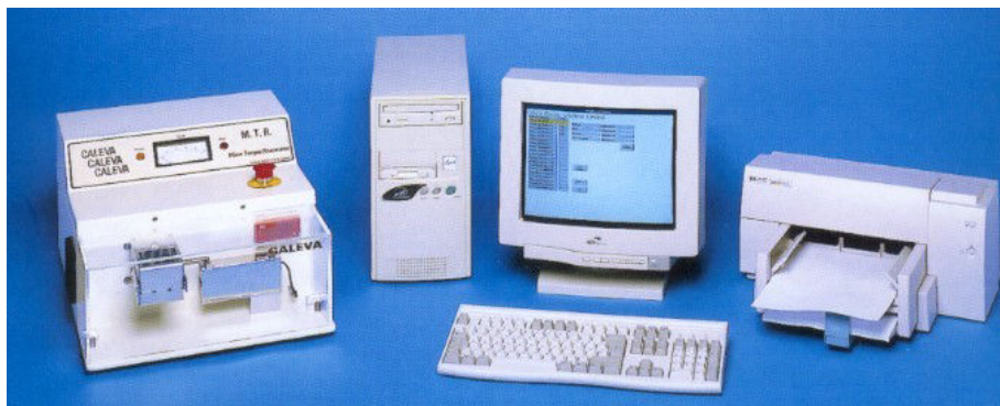
Figure 38 . Mixer Torque Rheometer (MTR)
