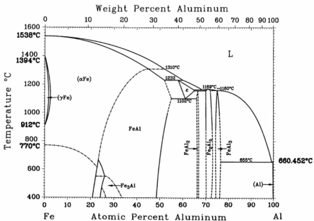
Figure IV- 3 – Diagramme de phase binaire Fe-Al [KUB1982].
