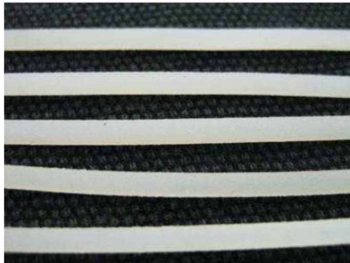
Figure 3.19 Extrudates of the UHMWPE/PP (50/50) blend mixed for 15 mins.
