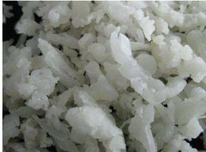
Figure 3.18 Extrudates of the UHMWPE/HDPE (50/50) blend.
