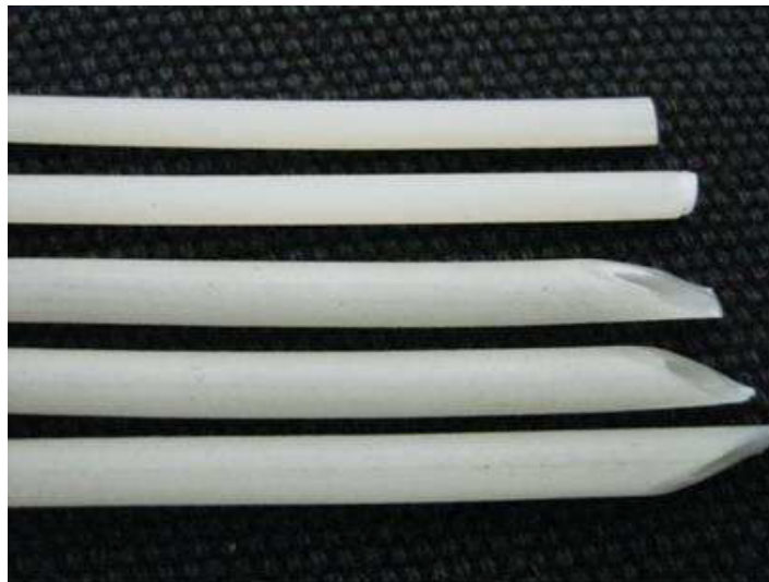
Figure 6.12 The bar and pipe of the UHMWPE/PP/PMM (90/10/5) composites.
