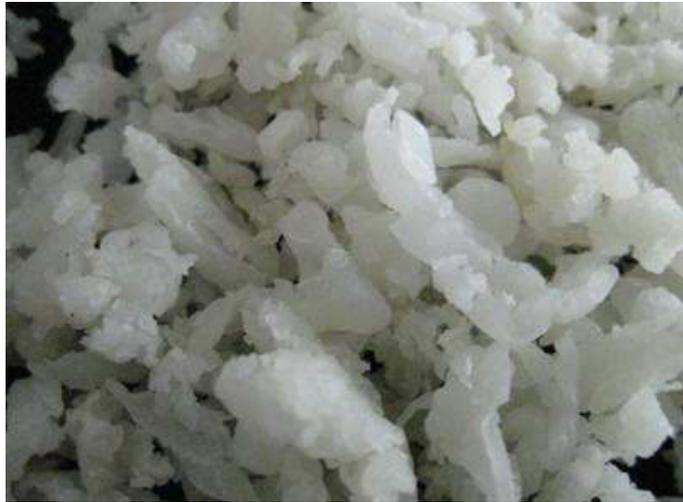
**Figure 3.18** Extrudates of the UHMWPE/HDPE (50/50) blend.
