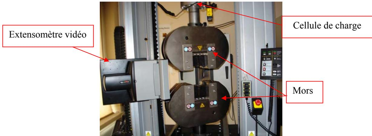
Figure III-2 : Machine de traction/compression INSTRON 5585H.
