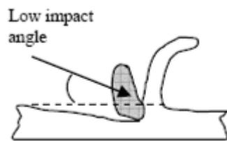
Figure I-3 : Erosion abrasive [10].
