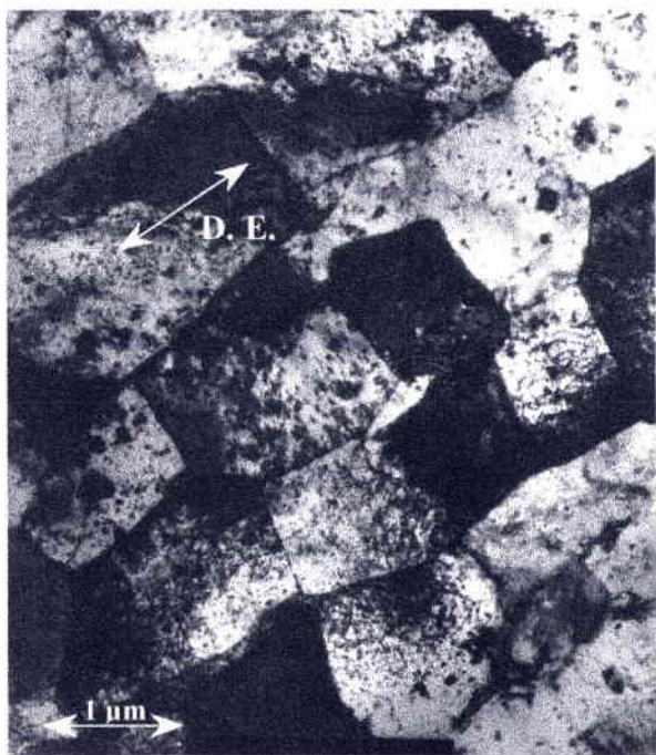
Fig. III.2-2 : Extrusion 1100°C, E.R. = 28 :1. (x15000)
