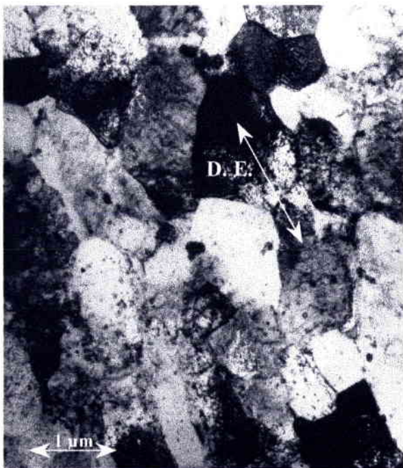
Fig. III.2-1 : Extrusion 1100°C, E.R. = 14 :1. (x15000)
