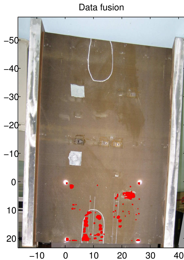
Figure 7.8: Representation of the defect area on a rectified live image taken with a digital camera.
