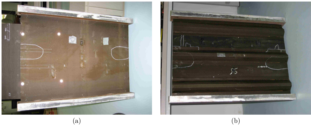
Figure 7.1: Image of the CFRP stiffened panel (a) from the front side (b) from the rear side (Component IV).
