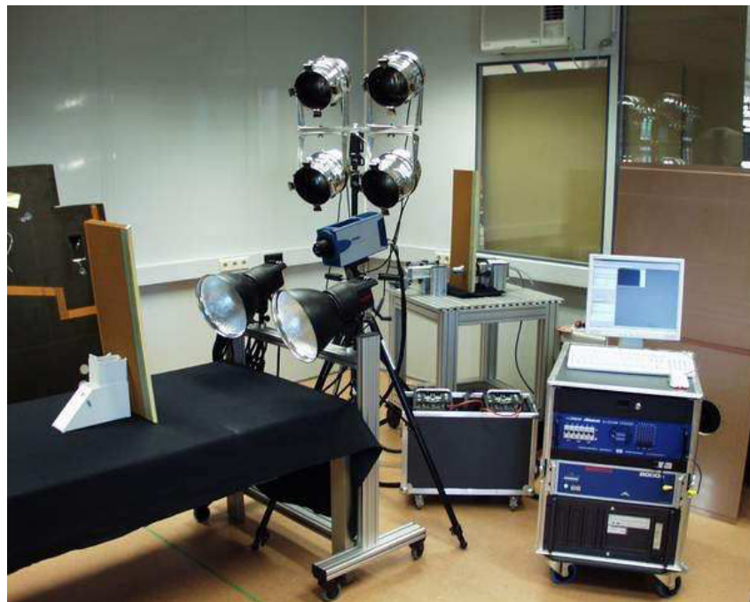
Figure 5.2: Thermography set-up of the Edevis company.
