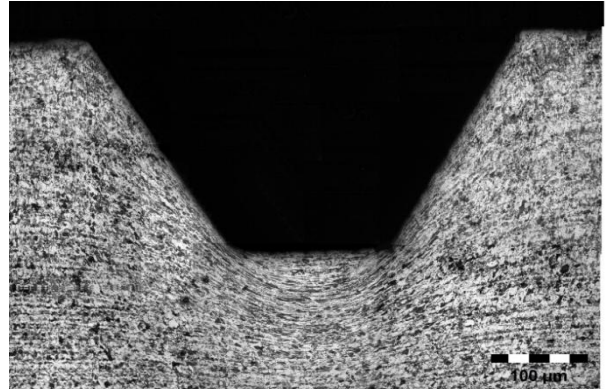
M20 - 18MnCr11 /p=36[bar]/n=1600[tours/min]
