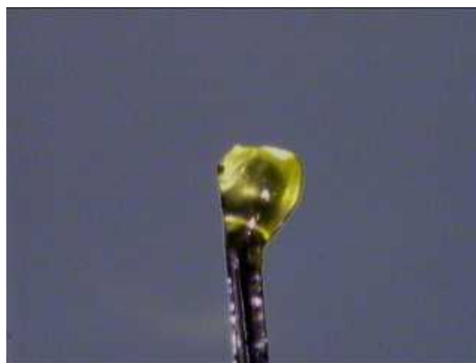
Figure 1.15: Image of the crystal of IV used in experiment. The crystal is mounted on a glass needle.
