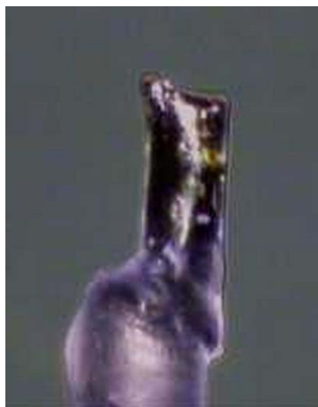
Figure 3.1.1: Frozen crystal of (VI) shown as mounted on goniometer during data collection.
