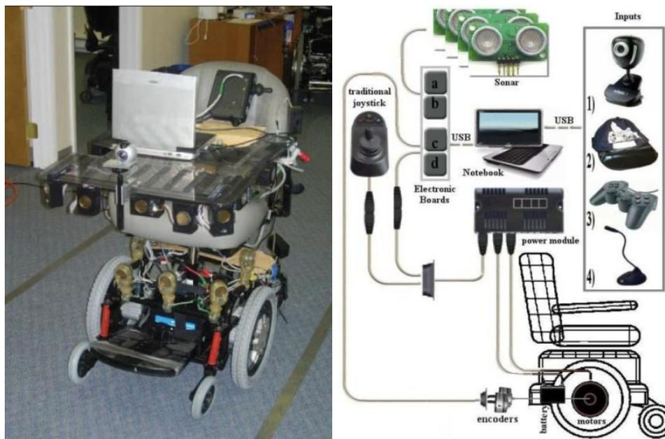
Fig. 1.2 : SWCS (a), Architecture IntellWheels (b).
