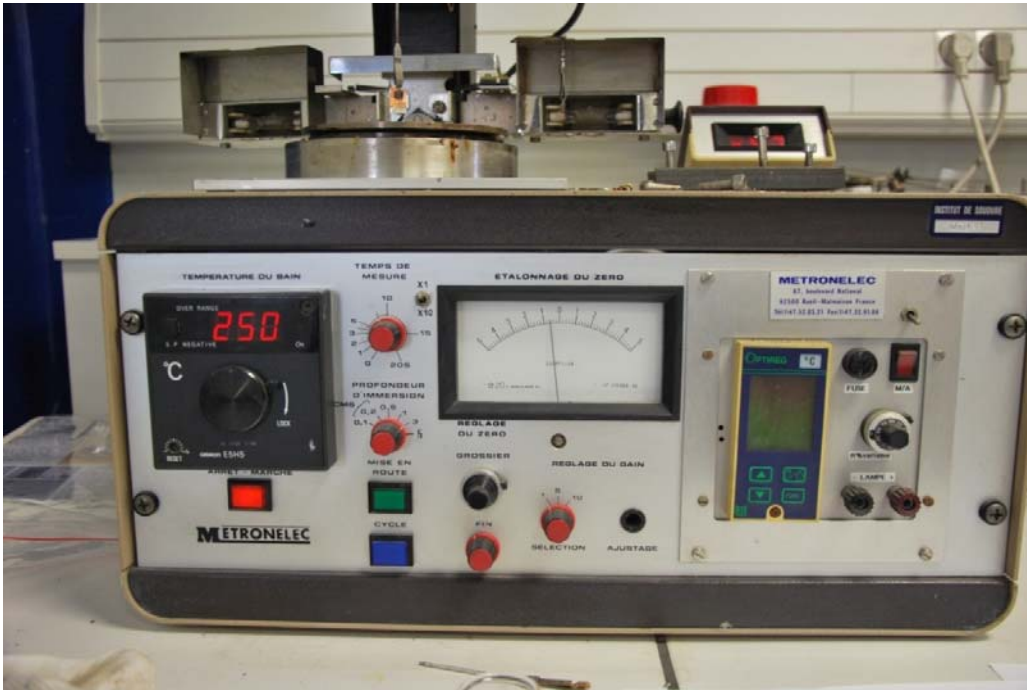
Figure 9.7: METRONELEC wettability setup
