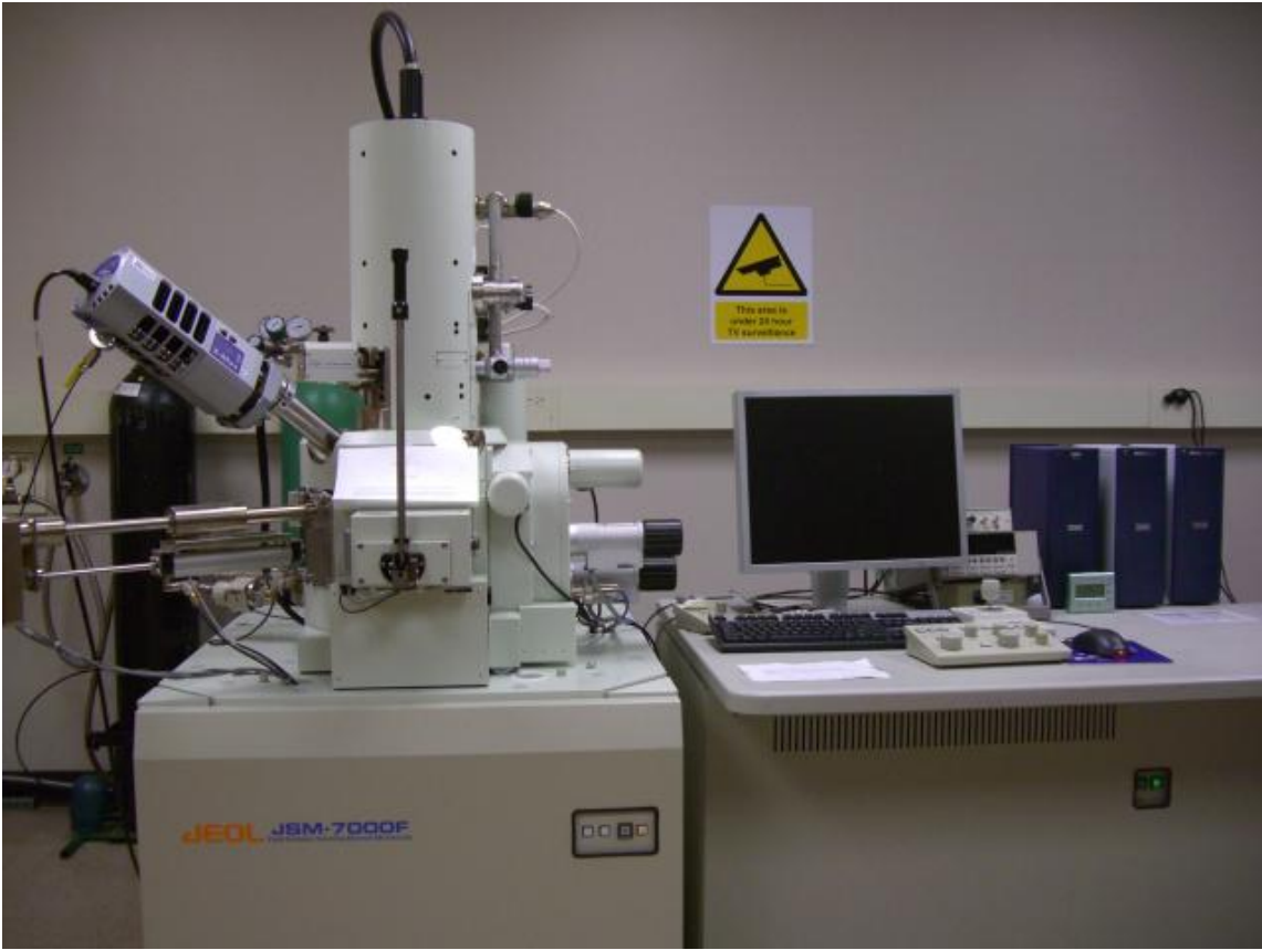
Figure 3.9: JEOL JSM-7000F Field Emission SEM
