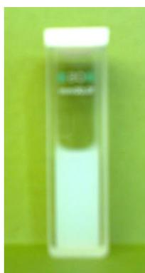
**Figure 1.2-6: Photo de solution de ZnO/P18Et2/MEK 1mg/1mg/ml illustrant sa stabilisation.**
