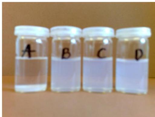
**Figure 7: Alumina suspensions after ultrasonication 30min (A) pH<sub>2</sub>, H<sub>2</sub>SO<sub>4</sub> ; (B) pH 2, HNO<sub>3</sub>; (C) KNO<sub>3</sub> 0.01M; (D) pH 2, HNO<sub>3</sub>, KNO<sub>3</sub> 0.01M.**
