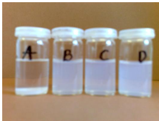
Figure 7: Alumina suspensions after ultrasonication 30min (A) pH 2 , H 2 SO 4 ; (B) pH 2, HNO 3 ; (C) KNO 3 0.01M; (D) pH 2, HNO 3 , KNO 3 0.01M.
