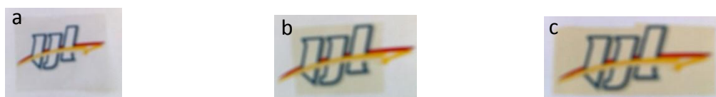
Figure 4: Digital images of (a) pure P(VDF-TrFE), (b) P(VDF-TrFE)/5wt.% \text{Al}_2\text{O}_3 and (c) P(VDF-TrFE)/10wt.% \text{Al}_2\text{O}_3 films.
