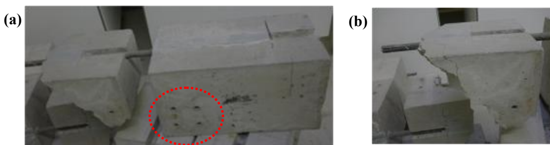
Fig. 3.48. Shear failure in the area of plate connector
