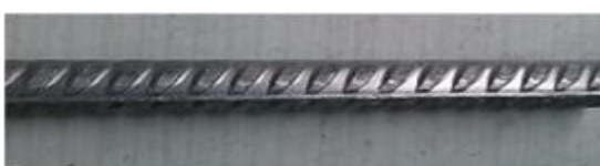
Fig. 3.1. Inoxydable steel reinforcement bar used (a) Austenitic-hot, (b) Austenitic-cold
