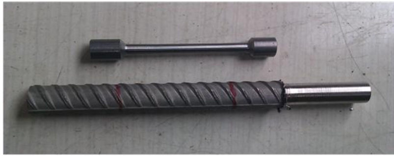
Fig. 3.2. Sample prepared for each of the inoxydable steel re-bar
