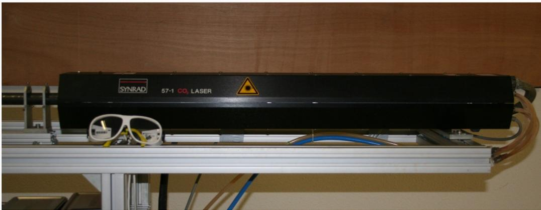
**Figure 5.5** – Laser CO<sub>2</sub> Continu de classe IV (130W)
