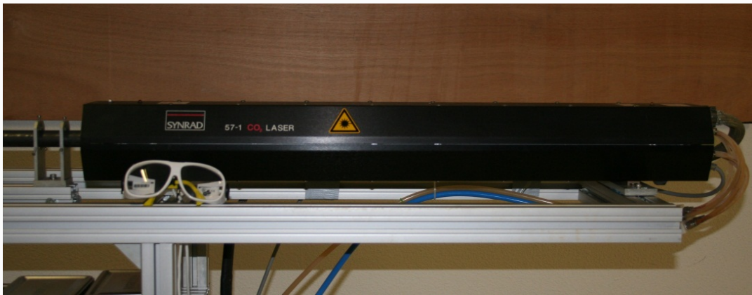
Figure 5.5 – Laser CO 2 Continu de classe IV (130W)
