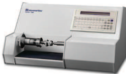
Figure 32 The illustration of GeoPyc 1360 envelope density analyser
