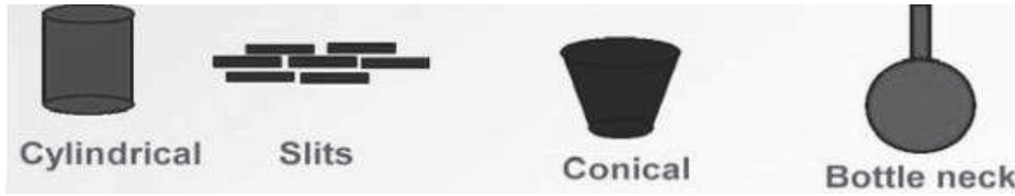
Figure 23 Different pore shapes in activated carbon [103]
