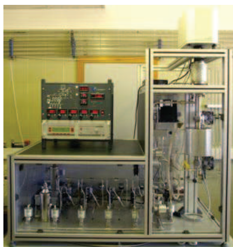
Figure 43 Determination of H 2 storage carried out with a gravimetric device at ICB (Zaragoza, Spain)
