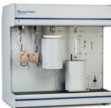
Figure 33 The illustration of ASAP 2020 automatic adsorption apparatus
