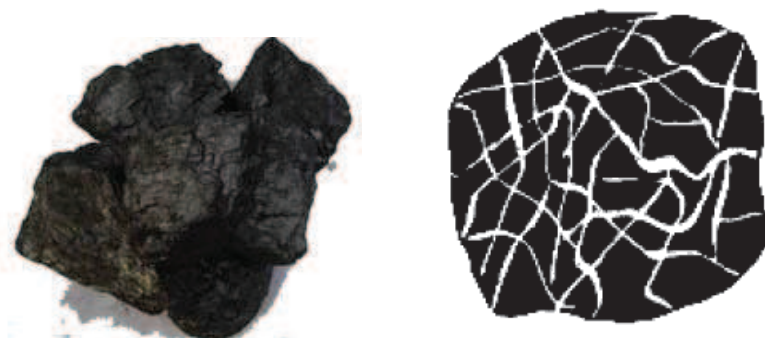
Figure 12 Raw carbon material (anthracite) on the left schematically transforms into the carbon on the right after activation [57]
