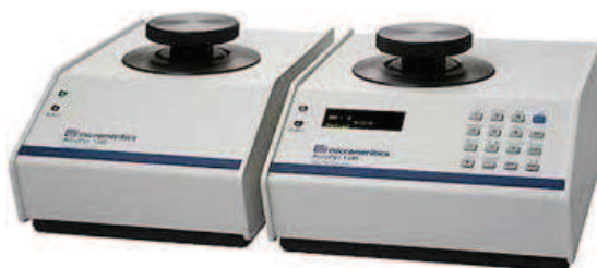
Figure 31 The illustration of Accupyc II 1340 Helium pycnometer
