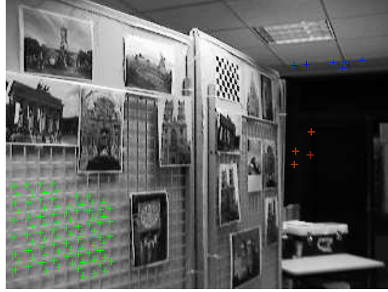
Figure 3.15: SIFT features belonging to the three largest clusters (marked by '+' in green, blue and red). Clusters are computed by range based transitive closure method on TD1 with T 125.
