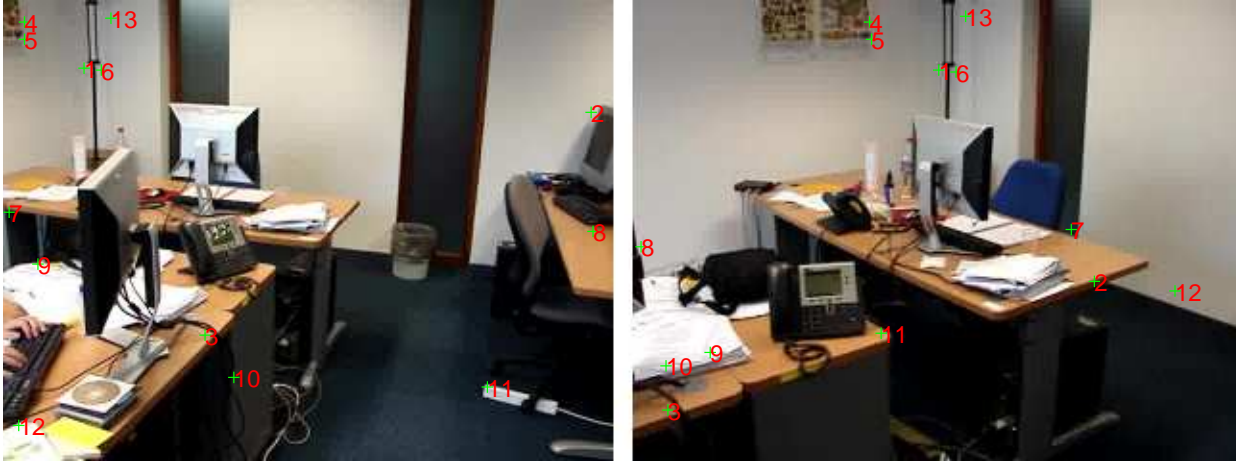
Figure 3.5: Points matched between frame 1 and 90 for r=250 . Total 13 matches. Matches numbered 2, 7, 8, 9, 10, 11 and 12 are incorrect.
