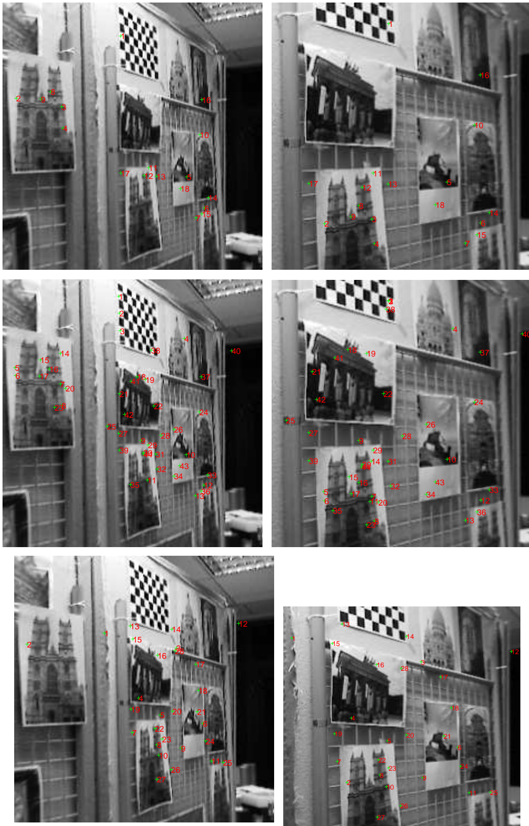
Figure 3.17: Comparing 2D-to-2D matches : The first two rows show the matches through standard SIFT keypoint matching with threshold 0.6 and 0.7 respectively. The last row shows the matches produced through ATC.
