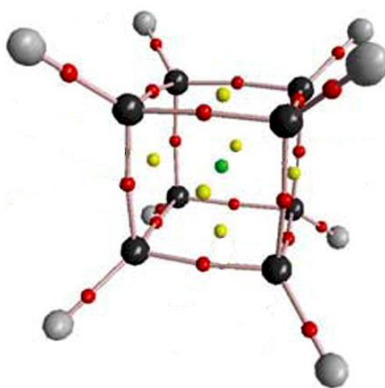
Figure I.5 Representation of the four possible critical points with rank three on an example of cubane molecule (C atom as black spheres, hydrogen as grey spheres): CCP – green, RCP – yellow, BCP – red, NCP – black at the nuclei position. 31
