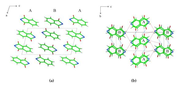
**Figure III.14** Crystal structure of C<sub>8</sub>H<sub>4</sub>O<sub>2</sub>Se. (a) Side view of the alternating columns A and B projected on the *ac*-plane; (b) down view of the A and B columns projected on the *bc*-plane. Intercolumn hydrogen bonding interactions are noted in red lines, chalcogen bondings are in blue lines.
