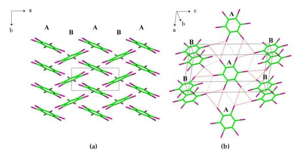
**Figure III.4** Crystal structure of C<sub>6</sub>Br<sub>6</sub>. (a) Side view of the alternating columns A and B projected in the *ab*-plane; (b) down view of the A and B columns projected in the *ac* plane. Intercolumn Hal<sub>3</sub>-synthon interactions are noted in red lines, while single Hal···Hal contacts are shown in grey. The columns are defined by symmetry operations (excluding lattice translations and inversion inside a molecule): A (x, y, z) and B (–x, 1/2+y, 1/2-z).
