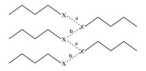
**Figure II.11** Schematic drawing of a zigzag (a = b) or ladder (a  $\ll$  b) type arrangement of the chalcogen …chalcogen interaction in the solid state (X = S, Se, Te).<sup>107a</sup>
