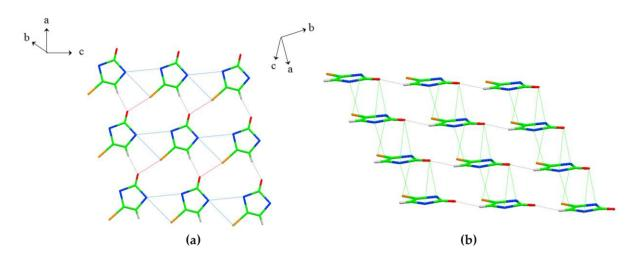
**Figure III.18** Crystal structure of C<sub>3</sub>HIOS<sub>2</sub>. (a) Down view on the sheet in *bc* plane. (b) Side view of the sheets in the *ac* plane. Hydrogen, halogen, and chalcogen intracolumn interactions are displayed in red (I··O), grey (H··O), and green (S···S, S···I). Intracolumn interactions are noted in blue.
