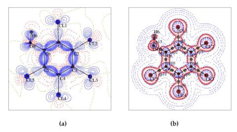
**Figure III.9** (a) Static deformation density  $\Delta \rho(\mathbf{r})$  and (b) negative Laplacian maps  $L(\mathbf{r})$  for the experimental multipolar model of C<sub>6</sub>Cl<sub>5</sub>OH drawn in the plane of the molecule.  $\Delta \rho(\mathbf{r})$  contours are at ±0.05 eÅ<sup>-3</sup> level: full lines in blue – positive, dotted lines in red – negative.  $L(\mathbf{r})$  contours (eÅ<sup>-5</sup>) are in logarithmic scale, red – positive, blue – negative.
