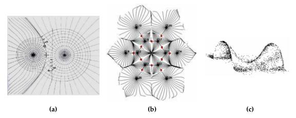
**Figure I.6** (a)  $\rho(\mathbf{r})$  contour map of NaCl overlaid with trajectories of  $\nabla \rho(\mathbf{r})$ . (b)  $\nabla \rho(\mathbf{r})$  for the chloranil molecule. The BCP's are marked in red. (c)  $\rho(\mathbf{r})$  exhibits a saddle distribution around the BCP and a local maximum at each nucleus.<sup>2</sup>
