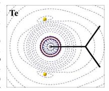
**Figure V.4**  $L(\mathbf{r}) = -\nabla^2 \rho(\mathbf{r})$  map of Te-atom in Te(CH<sub>3</sub>)<sub>2</sub> (plane bisecting the  $\alpha$ (C-Te-C) angle).  $L(\mathbf{r})$  contours (eÅ<sup>-5</sup>) are in logarithmic scale, red – positive, blue – negative. (3,–3) CPs (CC sites) are marked in yellow.
