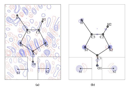
**Figure III.15** Residual electron density maps for C<sub>3</sub>HIOS<sub>2</sub> drawn in the plane of the molecule and in the two perpendicular planes bisecting the C–S–C angles: (a) experimental and (b) theoretical models. Contours are at ±0.05 eÅ<sup>-3</sup> level: full lines in blue – positive, dotted lines in red – negative. Resolution range is  $0 \le (\sin \theta/\lambda) \le 0.9$  Å<sup>-1</sup>.
