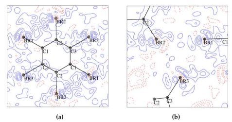
**Figure III.1** Residual electron density maps for the experimental model of C<sub>6</sub>Br<sub>6</sub> (synchrotron radiation) drawn (a) in the plane of the molecule and (b) in the plane of the Br<sub>3</sub>-synthon. Contours are at  $\pm$  0.05 eÅ<sup>-3</sup> level: full lines in blue – positive, dotted lines in red – negative. Resolution range is  $0 \le (\sin \theta/\lambda) \le 0.9$  Å<sup>-1</sup>.
