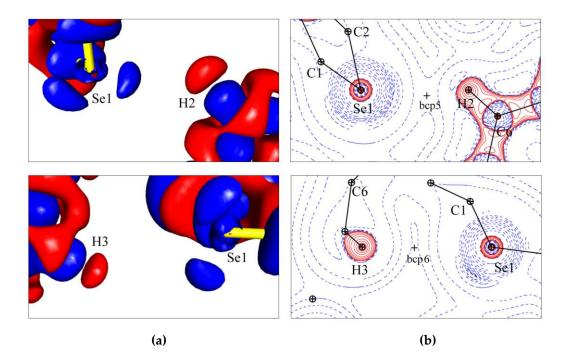
**Figure VI.6** Experimental maps in the intermolecular space of the hydrogen bonding in C<sub>8</sub>O<sub>2</sub>H<sub>4</sub>Se: (a) 3D static deformation density maps  $\Delta \rho(\mathbf{r})$ , iso-surface are drawn at 0.05 eÅ<sup>-3</sup>, blue – positive, red – negative; (b)  $L(\mathbf{r})$  contours (eÅ<sup>-5</sup>) are in logarithmic scale, red – positive, blue – negative.
