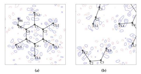
**Figure III.8** Residual electron density maps for the experimental model of C<sub>6</sub>Cl<sub>5</sub>OH drawn (a) in the plane of the molecule and (b) in the plane of the Cl<sub>3</sub>-synthon. Contours are at ±0.05 eÅ<sup>-3</sup> level: full lines in blue – positive, dotted lines in red – negative. Resolution range is  $0 \le (\sin \theta/\lambda) \le 0.9$  Å<sup>-1</sup>.
