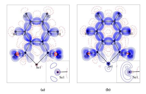
**Figure III.12** Static deformation density  $\Delta \rho(\mathbf{r})$  maps for C<sub>8</sub>H<sub>4</sub>O<sub>2</sub>Se drawn in the plane of the molecule and in a perpendicular plane bisecting the C–Se–C angle: (a) experimental and (b) theoretical models. Contours are at ±0.05 eÅ<sup>-3</sup> level: full lines in blue – positive, dotted lines in red – negative.
