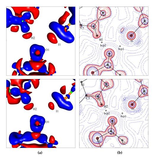
**Figure VI.4** Experimental (top) and theoretical (bottom) maps in the intermolecular space of the competing halogen (O…H) and hydrogen (O…I) bondings in the crystal structure of C<sub>3</sub>HIOS<sub>2</sub>: (a) 3D static deformation density maps  $\Delta \rho(\mathbf{r})$ , iso-surface are drawn at ±0.05 eÅ<sup>-3</sup>, blue – positive, red – negative; (b)  $L(\mathbf{r})$  maps, contours (eÅ<sup>-5</sup>) are in logarithmic scale, red – positive, blue – negative.
