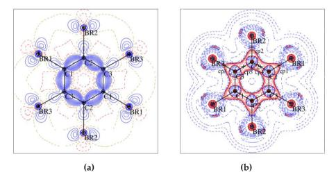
**Figure III.3** (a) Static deformation density  $\Delta \rho(\mathbf{r})$  and (b) negative Laplacian  $L(\mathbf{r})$  maps for the theoretical multipolar model of C<sub>6</sub>Br<sub>6</sub> drawn in the plane of the molecule.  $\Delta \rho(\mathbf{r})$  contours are at ±0.05 eÅ<sup>-3</sup> level: full lines in blue – positive, dotted lines in red – negative.  $L(\mathbf{r})$  contours (eÅ<sup>-5</sup>) are in logarithmic scale, red – positive, blue – negative.
