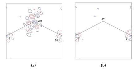
**Figure I.4** Residual density maps of the complex with zinc(II): (a) harmonic refinement, (b) anharmonic refinement.  $0.8 < \sin\theta/\lambda < 1.1 \text{ Å}^{-1}$ . Contours are at ±0.1 eÅ<sup>-3</sup> level: blue – positive, red – negative.<sup>27b</sup>
