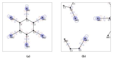
**Figure III.2** Residual electron density maps for the theoretical model of C<sub>6</sub>Br<sub>6</sub> drawn (a) in the plane of the molecule and (b) in the plane of the Br<sub>3</sub>-synthon. Contours are at ±0.05 eÅ<sup>-3</sup> level: full lines in blue – positive, dotted lines in red – negative. Resolution range is  $0 \le (\sin \theta/\lambda) \le 0.9$  Å<sup>-1</sup>.
