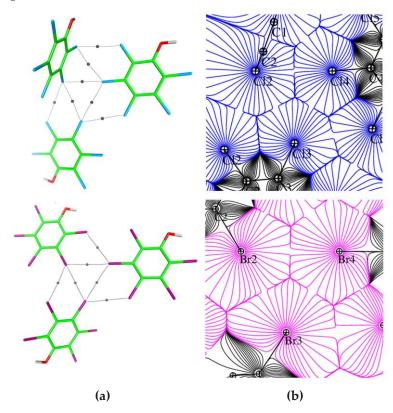
**Figure IV.1** Geometrical representation and  $\nabla \rho(\mathbf{r})$  map for the two types of synthons in (a) C<sub>6</sub>Br<sub>5</sub>OH (C<sub>6</sub>Cl<sub>6</sub> and C<sub>6</sub>Br<sub>6</sub> show a similar arrangement) and (b) C<sub>6</sub>Cl<sub>5</sub>OH. The BCP's corresponding to type-II Hal···Hal interactions in synthons, along with those of the accompanying type-I Hal···Hal contacts are represented as grey points.
