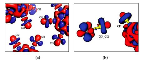
**Figure II.5** 3D static deformational density maps  $\Delta\rho(\mathbf{r})$  representing (a) three Type-II Cl…Cl interactions forming a synthon and three Type-I Cl…Cl interactions in C<sub>6</sub>Cl<sub>6</sub>, iso-surfaces are drawn at ±0.05 eÅ<sup>-3</sup> level<sup>83</sup> (b) Type-II interaction in 2-chloro-3-chloromethyl-8-methylquinoline.<sup>89</sup> Iso-surfaces are drawn at ±0.01 eÅ<sup>-3</sup> level. Blue – positive, red – negative.
