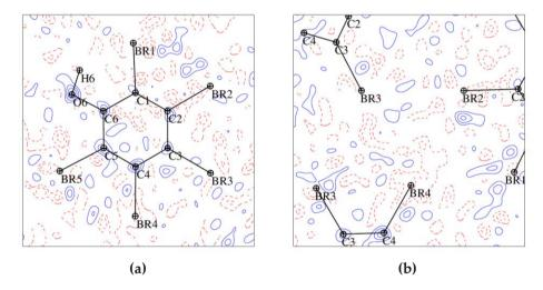
**Figure III.5** Residual electron density maps for the experimental model of C<sub>6</sub>Br<sub>5</sub>OH drawn (a) in the plane of the molecule and (b) in the plane of the Br<sub>3</sub>-synthon. Contours are at ±0.05 eÅ<sup>-3</sup> level: full lines in blue – positive, dotted lines in red – negative. Resolution range is  $0 \le (\sin \theta/\lambda) \le 0.9$  Å<sup>-1</sup>.
