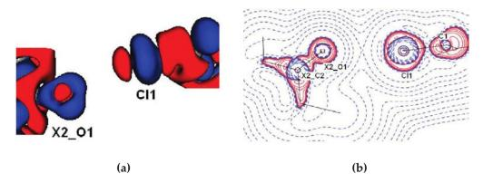
**Figure II.7** (a) 3D static deformational density and (b)  $L(\mathbf{r})$  maps representing an electrostatically attractive  $Cl(\delta/CD)\cdots O(\delta/CC)$  interaction. Iso-surface of  $\Delta\rho(\mathbf{r})$ at ±0.05 eÅ<sup>-3</sup>, blue – positive, red – negative ;  $L(\mathbf{r})$  contours (eÅ<sup>-5</sup>) are in logarithmic scale, red – positive, blue – negative <sup>94</sup>
