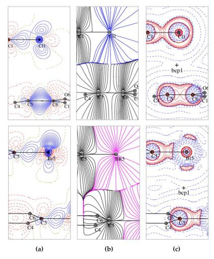
**Figure IV.8** Intermolecular interactions Cl<sub>1</sub>···C<sub>5</sub> in C<sub>6</sub>Cl<sub>5</sub>OH (top) and Br<sub>5</sub>···C<sub>5</sub> in C<sub>6</sub>Br<sub>5</sub>OH (bottom): (a) static deformation density maps, contours are at ±0.05 eÅ<sup>-3</sup>, blue – positive, red – negative, (b)  $\nabla \rho(\mathbf{r})$  map and (c)  $L(\mathbf{r})$  maps, contours (eÅ<sup>-5</sup>) are in logarithmic scale, red – positive, blue – negative.
