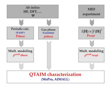
Figure I.1 Scheme illustrating chemical bond characterization, based on electron density function, determined theoretically or experimentally and analyzed with QTAIM approach.
