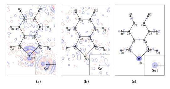
**Figure III.11** Residual electron density maps for C<sub>8</sub>H<sub>4</sub>O<sub>2</sub>Se drawn in the plane of the molecule and in the perpendicular plane bisecting the C–Se–C angle: (a) experimental (synchrotron), (b) experimental (Mo K $\alpha$ ) and (c) theoretical models. Contours are at ±0.05 eÅ<sup>-3</sup> level: full lines in blue – positive, dotted lines in red – negative. Resolution range is  $0 \le (\sin \theta / \lambda) \le 0.8$  Å<sup>-1</sup>.
