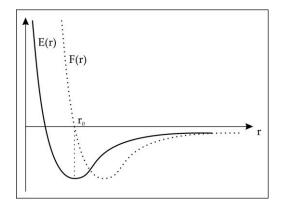
**Figure I.12** A typical potential energy curve (in arbitrary units) versus internuclear separation  $\mathbf{r} \ E(\mathbf{r})$  for a diatomic system superposed with force function  $F(\mathbf{r})$ . At the equilibrium distance, the attractive and repulsive components of force are equal.
