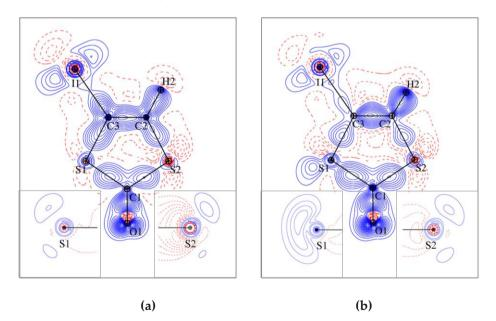
**Figure III.16** Static deformation density  $\Delta \rho(\mathbf{r})$  maps for C<sub>3</sub>HIOS<sub>2</sub> drawn in the plane of the molecule and in the two perpendicular planes bisecting the C–S–C angles: (a) experimental and (b) theoretical models. Contours are at ±0.05 eÅ<sup>-3</sup> level: full lines in blue – positive, dotted lines in red – negative.
