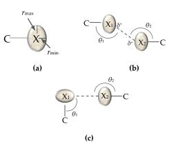
**Figure II.2** (a) Anisotropic distribution of  $\rho(\mathbf{r})$  around halogen atom (X), showing different atomic radii ( $r_{min}/r_{max}$ ) along polar and equatorial directions (b) Type-I interaction ( $\theta_1 \approx 90^\circ$ ,  $\theta_2 \approx 180^\circ$ ). <sup>61</sup>
