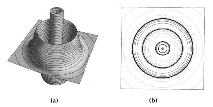
**Figure I.10** (a) Truncated version of the relief map of  $L(\mathbf{r}) = -\nabla^2 \rho(\mathbf{r})$  function and (b) the corresponding contour map for a spherically symmetric electron density of an isolated Ar-atom.<sup>2</sup> Contours (eÅ<sup>-5</sup>) are in logarithmic scale.
