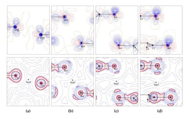
**Figure IV.7** Static deformation density (top) and  $L(\mathbf{r})$  maps (bottom) for Type-I Hal…Hal interactions (a) *head-on* and (b), (c), (d) the variations of *side-side* geometrical arrangements.  $\Delta \rho(\mathbf{r})$  contours are at ±0.05 eÅ<sup>-3</sup>, blue – positive, red – negative;  $L(\mathbf{r})$  contours (eÅ<sup>-5</sup>) are in logarithmic scale, red – positive, blue – negative.
