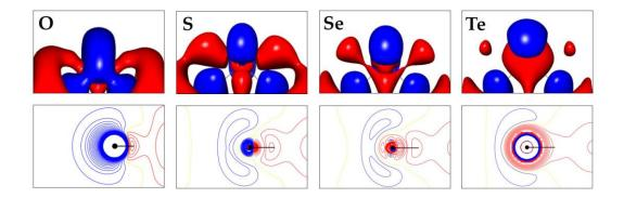
**Figure V.1** Deformation density  $\Delta\rho(\mathbf{r})$  maps around chalcogen atoms in C<sub>8</sub>O<sub>2</sub>H<sub>4</sub>Chal monomers (C-Chal-C plane (top) and perpendicular plane bisecting the  $\alpha$ (C-Chal-C) angle (bottom), obtained from gas-phase calculations. Iso-surfaces and contours are drawn at ±0.05 eÅ<sup>-3</sup> levels: blue – positive, red – negative.
