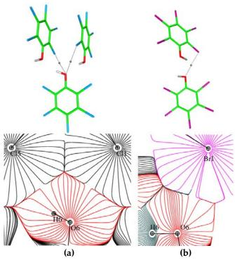
**Figure V.11** Intermolecular interactions involving O-atoms in the crystal structures of (a) C<sub>6</sub>Cl<sub>5</sub>OH (O<sub>6</sub>···Cl<sub>1</sub>/Cl<sub>5</sub>) and (b) C<sub>6</sub>Br<sub>5</sub>OH (O<sub>6</sub>···Br<sub>1</sub>), represented by the bond paths and the corresponding BCP's between the interacting atoms (top) and by the gradient  $\nabla \rho(\mathbf{r})$  maps (bottom).
