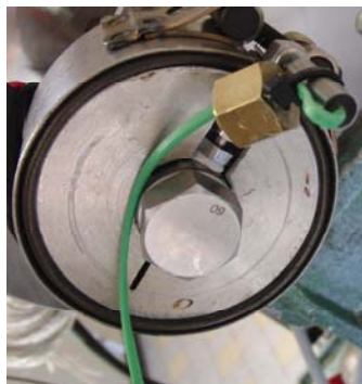
Fig.: 3.16 – Nozzle assembly with 60 \mu\text{m} nozzle, thermocouple and heating jacket.
