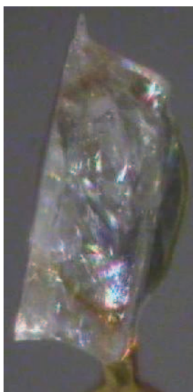
Figure 112. Crystal of IV placed in the mounting loop for measurement.
