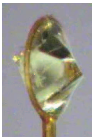
Figure 30. Crystal of I placed in the mounting loop for measurement.
