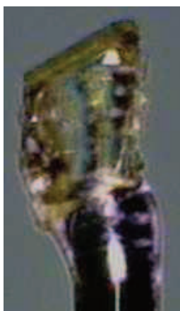
Figure 58. Crystal of II mounted on the top of the glass stirring rod.
