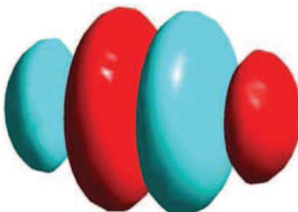
Figure 14. An example of the graphical representation of density modulation due to high-order terms in Gram-Charlier series expansion of a Gaussian atomic probability density function: b^{222} third order term in \bar{4} point group [reprinted from International Tables for Crystallography, vol. D].
