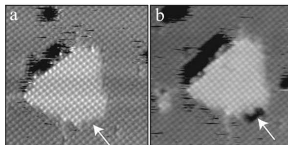
**Figure 5.**  $20 \text{ nm} \times 20 \text{ nm}$  high-resolution STM images acquired at 40-min interval at the same location ((a)  $V_b = -2.0 \text{ V}$ ,  $I_t = 0.19 \text{ nA}$ ; (b)  $V_b = -2.6 \text{ V}$ ,  $I_t = 0.05 \text{ nA}$ ). The overall shape of the triangular defect varies slightly with time. The arrow points to an area which displays an inverse contrast from one image to the next.
