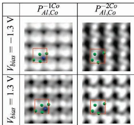
**Figure 10.** Simulated STM images of the two surface models  $P_{Al,Co}^{-1Co}$  and  $P_{Al,Co}^{-2Co}$  built from the bulk truncated  $P_{Al,Co}$  model. The simulated images are calculated with a tip–surface distance equal to 3 Å. One surface unit cell has been superimposed on the calculated STM images (the Al atoms are in gray (green) and the Co atoms in black (blue)).
