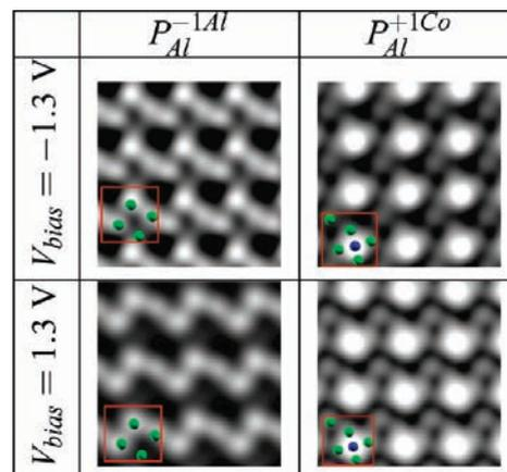
**Figure 9.** Simulated STM images of the two surface models  $P_{Al}^{-1Al}$  and  $P_{Al}^{+1Co}$  built from the bulk truncated  $P_{Al}$  model. The simulated images are calculated with a tip–surface distance equal to 3 Å. One surface unit cell has been superimposed on the calculated STM images (the Al atoms are in gray (green) and the Co atoms in black (blue)).
