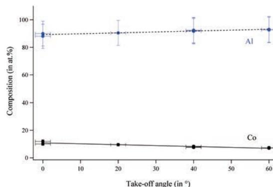
**Figure 2.** Variation of the elemental composition at the  $\text{Al}_9\text{Co}_2$  (001) surface as a function of the photoelectrons takeoff angle. The measurements at  $60^\circ$  are more surface sensitive than those performed at  $0^\circ$ . The solid (black) and dashed (blue) lines correspond to the Co and Al contents, respectively.
