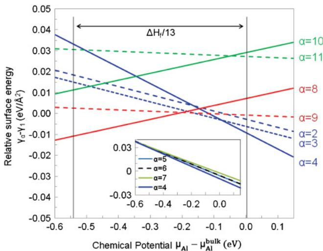
FIG. 5. (Color online) Relative surface energy (relative to model 1) vs the chemical potential  $\mu_{\text{Al}}$  for the 11 different surface models shown in Figs. 2–4. The inset shows magnified results for the surface model 4 and its derivatives (models 5, 6, and 7).
