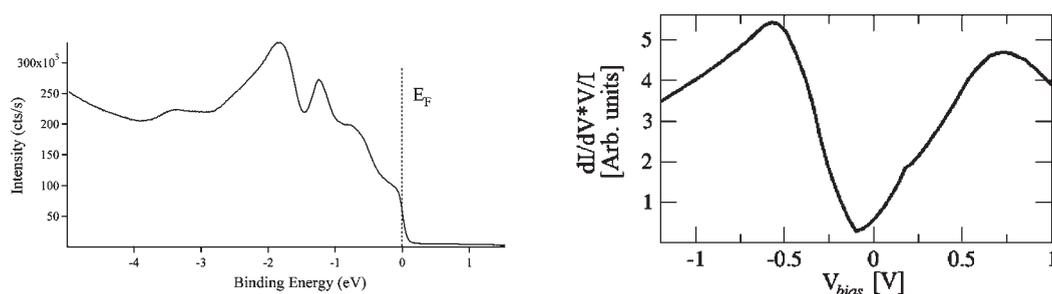
**Figure 3.** Left: Experimental UPS valence band spectrum of  $\text{Al}_3\text{Co}_2$  (001) surface up to 5 eV. The position of  $E_F$  is indicated by a dashed line. Right: Experimental STS spectrum.
