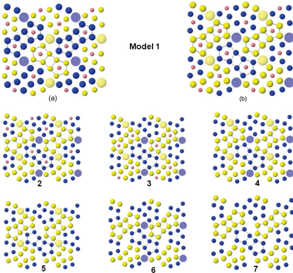
FIG. 2. (Color online) The model structures of complete  $P$ -layer termination. (a) and (b) show the two different  $P$  layers,  $P_1$  and  $P_2$ , indicating the bipentagon features. The models are numbered as described in the text. Small (pink) circles indicate the Co atoms, present only in models 1–3. The larger circles correspond to Al glue atoms. The remaining blue (yellow) circles correspond to Al atoms above (below) the center of mass of the  $P$  layer.
