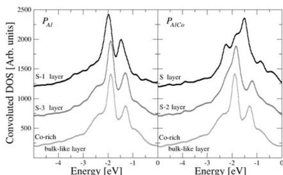
**Figure 14.** LDOS of the S-1 and S-3 surface atomic layers from the  $P_{Al}$  model (left) and S and S-2 layers from the  $P_{Al,Co}$  model (right) compared to the contribution of a similar layer in the bulk.
