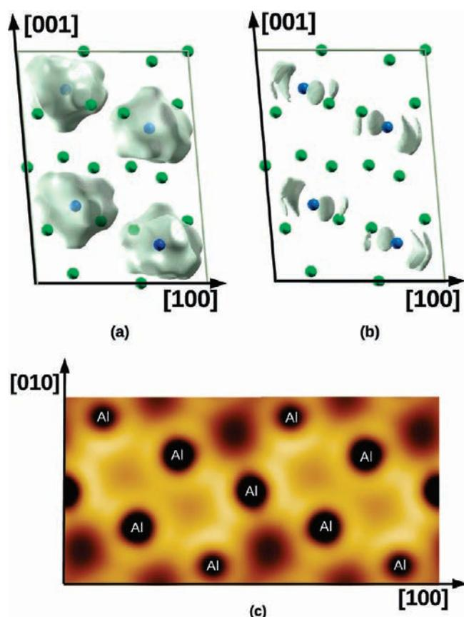
**Figure 13.** (a) Isodensity surface ( $0.28 \text{ \AA}^{-3}$ ) of the total charge density of bulk  $\text{Al}_9\text{Co}_2$ . (b) Isodensity surface ( $0.07 \text{ \AA}^{-3}$ ) of the difference between the total charge density and the superposition of atomic charge density. (c) Contour plot of the total electron density in the  $P_{\text{Al}}$  plane ( $12.40 \text{ \AA} \times 6.28 \text{ \AA}$ ,  $z = 0.5$ ).
