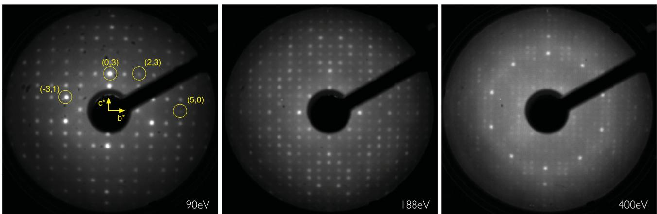
FIG. 8. (Color online) LEED patterns from  $\text{Al}_{13}\text{Co}_4$  at a sample temperature of  $80 \text{ K}$ , for beam energies  $90$ ,  $188$ , and  $400 \text{ eV}$ . The beam indices are indicated for selected beams.
