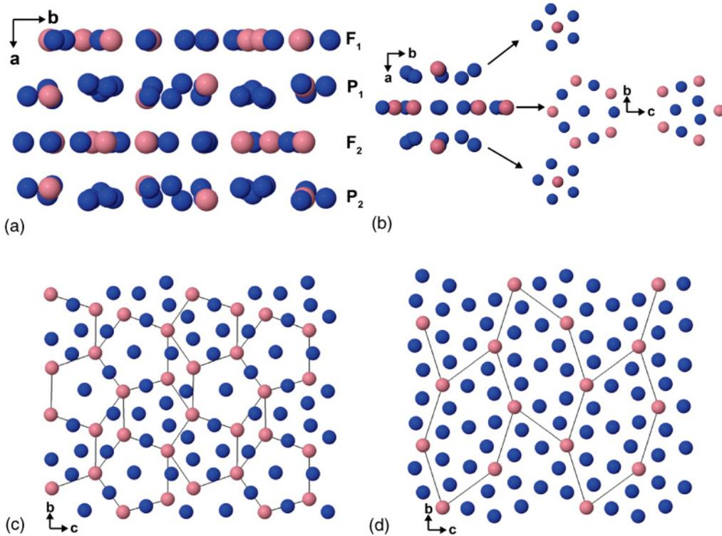
FIG. 1. (Color online) The bulk structure of  $\text{Al}_{13}\text{Co}_4$ . The dark (blue) spheres are aluminum and the light (pink) spheres are cobalt. (a) Side view of the unit cell, composed of four layers of atoms. (b) Side view (left) of the pyramid structure, and a top view (right) of each layer. The registry of the center  $F$  layer is different for  $F_1$  and  $F_2$ ; both are shown. (c) Top view of  $F$  layer. (d) Top view of  $P$  layer.
