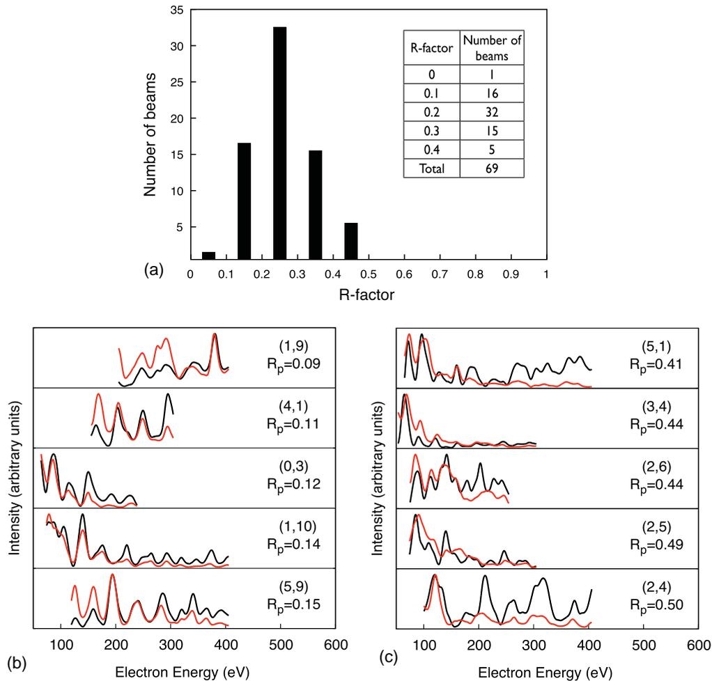
FIG. 10. (Color online) (a) Distributions of  $R$  factor for all beams in the best-fit structure. (b) best five beams, and (c) worst five beams of the experimental (black/bold) and best-fit calculated (red/light) LEED spectra, with individual  $R$  factors. The complete set of curves is given in the supplementary material (Ref. 35).
