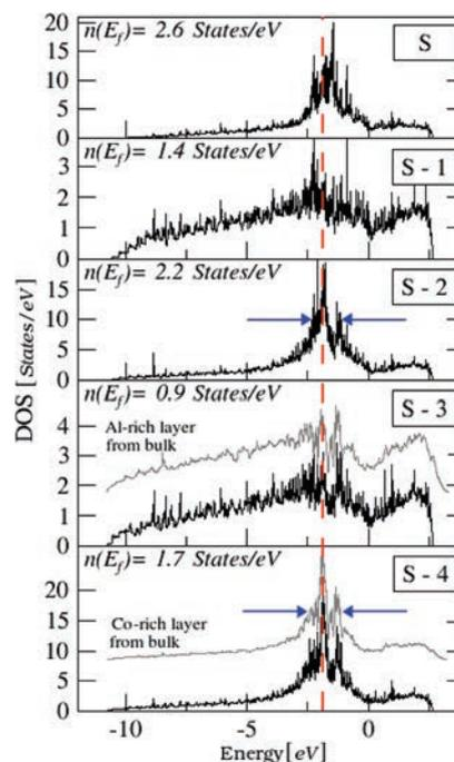
**Figure 12.** LDOS (black) of the  $P_{Al,Co}$  topmost layer. The topmost atomic layer is labeled S, the sublayers S–1, etc. The LDOS of the “S–3” and “S–4” layers are compared with the corresponding calculated LDOS of the bulk (gray)  $P_{Al}$  and  $P_{Al,Co}$  atomic planes, respectively. The vertical dashed (red) line points out the maximum of the “S–4” LDOS to give a reference point for its shifting. The (blue) arrows indicate the DOS value at which the band widths have been calculated.
