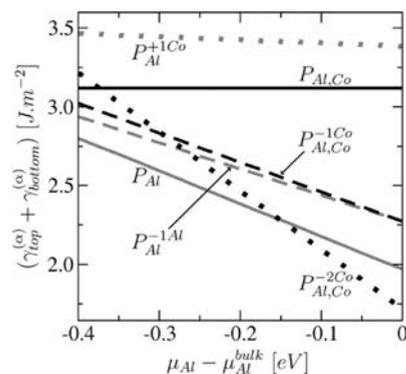
**Figure 7.** Surface energies  $\gamma_{\text{top}}^{(\alpha)} + \gamma_{\text{bottom}}^{(\alpha)}$  as a function of  $\Delta H_f/9 \leq \mu_{\text{Al}} - \mu_{\text{Al}}^{\text{Bulk}} \leq 0$ . Gray lines: the models derived from the  $P_{\text{Al}}$  model. Black lines: the models obtained from the  $P_{\text{Al,Co}}$  model (see text).
