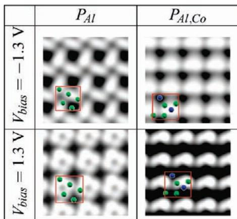
**Figure 8.** Simulated STM images of the two surface models  $P_{Al}$  and  $P_{Al,Co}$ . The simulated images are calculated with a tip–surface distance equal to 3 Å. One surface unit cell has been superimposed on the calculated STM images (the Al atoms are in gray (green) and the Co atoms in black (blue)).
