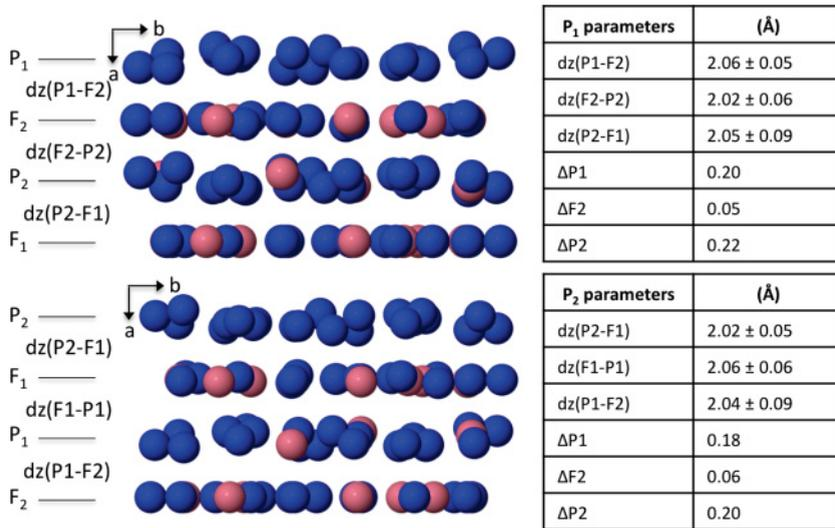
FIG. 9. (Color online) Relaxations of the surface layers of terminations  $P_1$  and  $P_2$  for the best-fit structure (4 in Table I). The  $dz$  parameters correspond to the average interlayer spacings, and the  $\Delta$  parameters correspond to the puckering amplitude for each layer.
