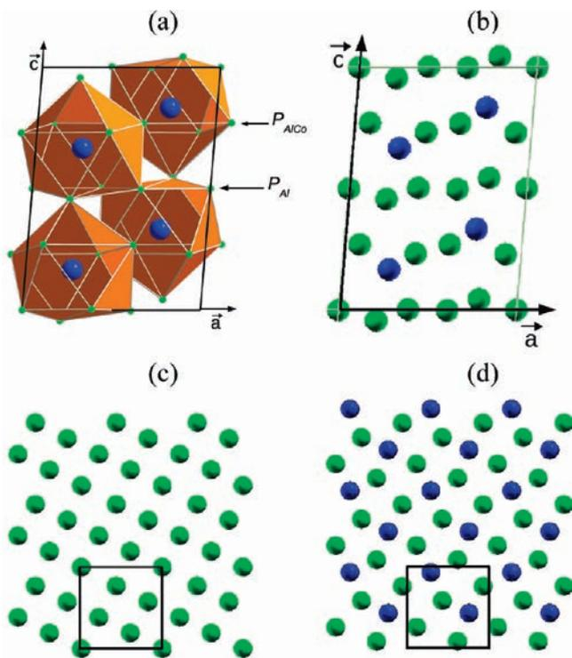
**Figure 6.**  $\text{Al}_9\text{Co}_2$  atomic structure. Gray (green) spheres correspond to Al atoms and black (blue) spheres to Co atoms. (a) Single-capped square antiprismatic clusters of the structure have been highlighted. (b) Structure projected along the [010] direction showing the sequence of two types of atomic layers in the structure. (c) (001) pure Al atomic plane ( $P_{\text{Al}}$ ). (d) (001) atomic plane containing both aluminum and cobalt atoms ( $P_{\text{Al,Co}}$ ).
