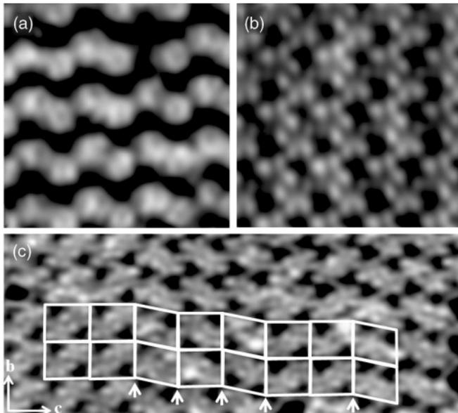
FIG. 6. STM images ( $6 \times 6 \text{ nm}^2$ ) of the (100) surface terminations of sample 1 [(a),  $V = -1.3 \text{ V}$ ] and of sample 2 [(b),  $V = -0.6 \text{ V}$ ]. (c) STM image ( $15 \text{ nm} \times 6 \text{ nm}$ ,  $V = -0.6 \text{ V}$ ) obtained on sample 2 showing twin planar defects in the (100) surface. A tiling is superimposed, with rectangular (orthorhombic) and oblique (monoclinic) cells. Arrows indicate domain boundaries.
