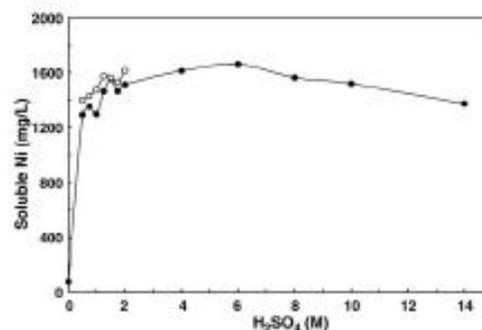
**Fig. 2.** Effect of sulphuric acid concentration on nickel solubilisation from *A. murale* seeds, leaching period = 120 min; solids concentration = 150 g/L; temperature = 90 °C. Symbols: (●) without  $H_2O_2$ , (○) with 4 g  $H_2O_2$ .
