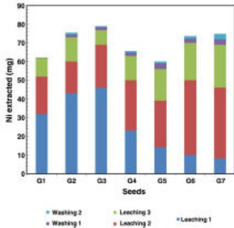
Fig. 3. Nickel extraction from *A. maritima* seeds during the counter-current leaching process. Leaching period = 120 min; solids concentration = 132 g/L; H<sub>2</sub>SO<sub>4</sub> concentration = 0.5 M; temperature = 90 °C.
