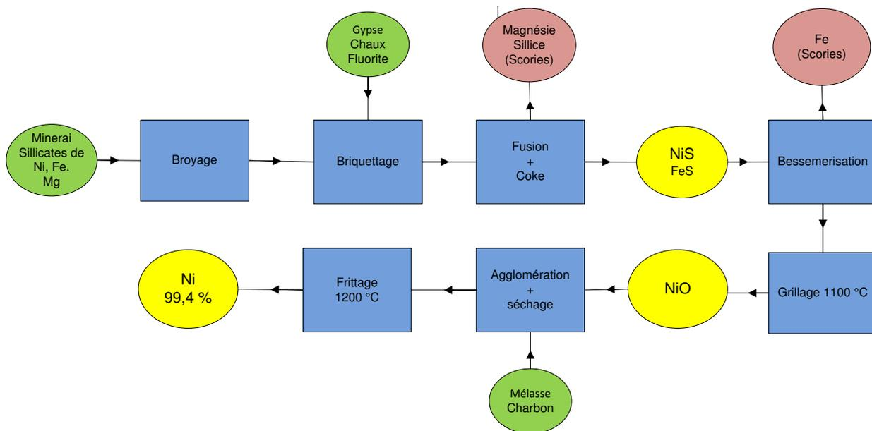
**Figure 1.9 Fusion sulfurante**
