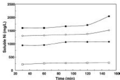
**Fig. 1.** Effect of total solid concentration on nickel solubilisation from *A. murale* seeds.  $H_2SO_4$  concentration = 14 M; temperature = 90 °C. Symbols: (●) 100 g/L, (○) 150 g/L, (■) 200 g/L, (□) 250 g/L.
