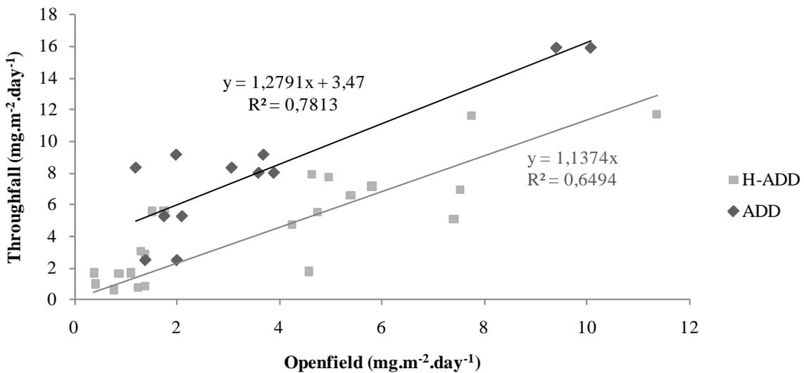
Figure 54: Daily deposition rates of ADD (dark gray) and H-ADD (light gray) in throughfall compared to those in openfield (mg.m<sup>-2</sup>.day<sup>-1</sup>) at the Montiers site. ADD is calculated as the difference between APD and POM, and POM is calculated from the C content in APD multiplied by the agronomic factor 1.72. H-ADD was sampled between April 2010 and March 2012 while ADD was measured from September 2011 to March 2012.
