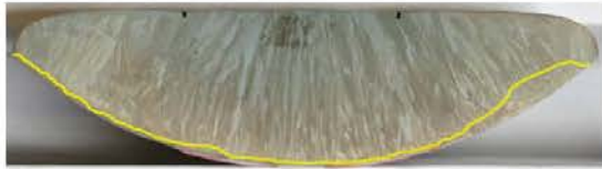
Fig. 4 Macrography of a sectioned button of nickel-based superalloy
