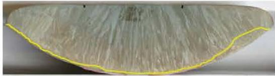
Fig. 4 Macrography of a sectioned button of nickel-based superalloy
