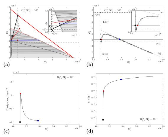
Figure 2.15: Results of the *u*-model (abscissae are  $u_{\rm C}^{\alpha}$ ) for  $D_{\rm X}^{\gamma*}/D_{\rm X}^{\gamma} = 10^4$ : (a) tie-lines; (b) nominal concentration  $u_{\rm X}^0$ ; (c) total dissipation; (d) growth rate.
