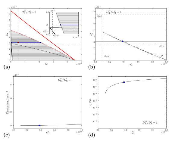
Figure 2.14: Results of the *u*-model (abscissae are  $u_{\rm C}^{\alpha}$ ) for  $D_{\rm X}^{\gamma*}/D_{\rm X}^{\gamma} = 1$ : (a) tie-lines; (b) nominal concentration  $u_{\rm X}^0$ ; (c) total dissipation; (d) growth rate.
