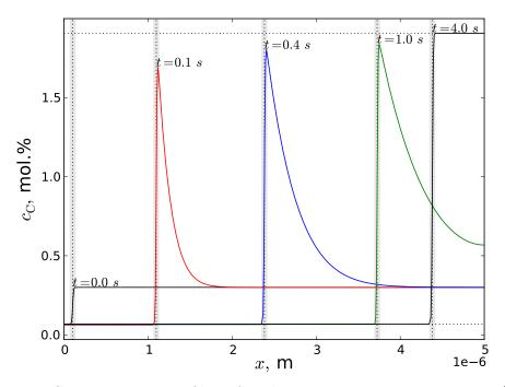
Figure 3.8: Concentration profiles of carbon at successive time steps (diffuse interface located by grey slabs).
