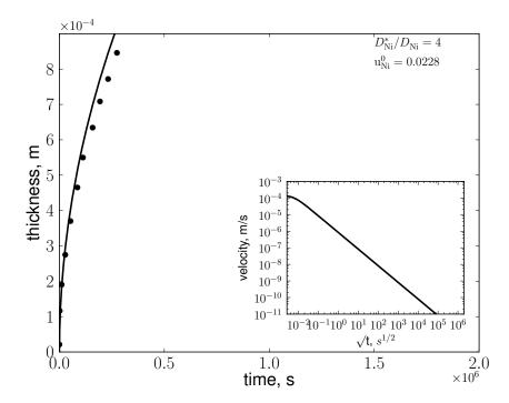
Figure 2.23: Ferrite growth kinetics in a Fe-0.5 at.%C-2.27 at.%Ni alloy at 700°C (inset: growth rate vs. time): present work (continous line) and results from [124] (dots).
