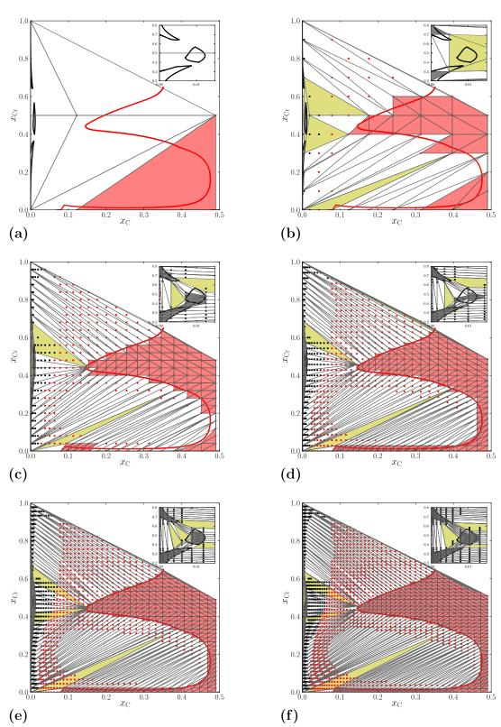
Figure 1.11: Projections of the final convex hulls (triangles) of the Gibbs energies of  $\alpha$  (black dots) and  $\gamma$  (red dots) in Fe-C-Cr at 600°C, for N = 2 (a), N = 10 (b), N = 25 (c), N = 35 (d), N = 45 (e) and N = 55 (f).
