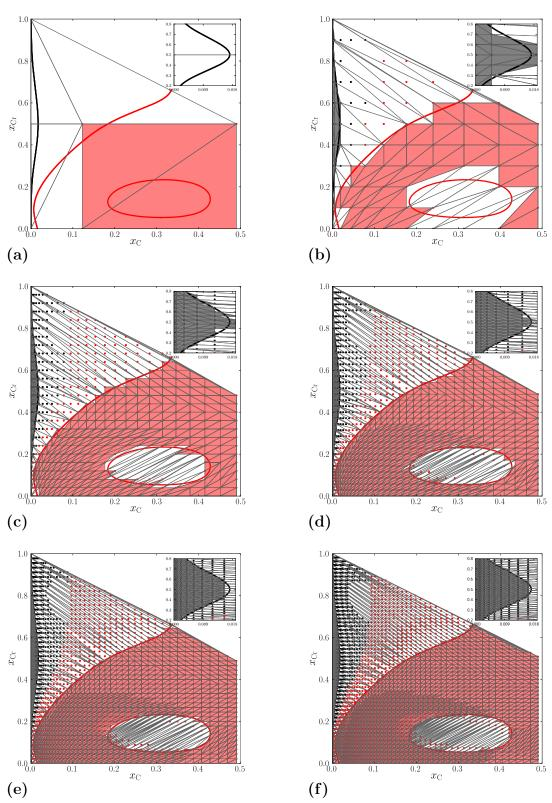
Figure 1.10: Projections of the final convex hulls (triangles) of the Gibbs energies of  $\alpha$  (black dots) and  $\gamma$  (red dots) in Fe-C-Cr at 800°C, for N = 2 (a), N = 10 (b), N = 25 (c), N = 35 (d), N = 45 (e) and N = 55 (f).
