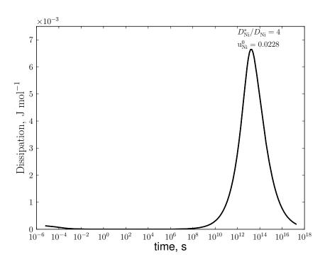
Figure 2.24: Evolution of the interfacial dissipation during growth of ferrite at 700°C in a Fe-0.5 at.%C-2.27 at.%Ni alloy.
