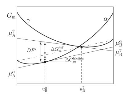
Figure 2.1: Additive contributions to the dissipation of the driving force at a moving  $\alpha/\gamma$  interface with concentrations  $u_{\rm B}^{\alpha}$  and  $u_{\rm B}^{\gamma}$  in an A-B binary alloy.
