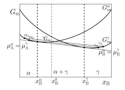
Figure 1.1: Common tangent construction.
