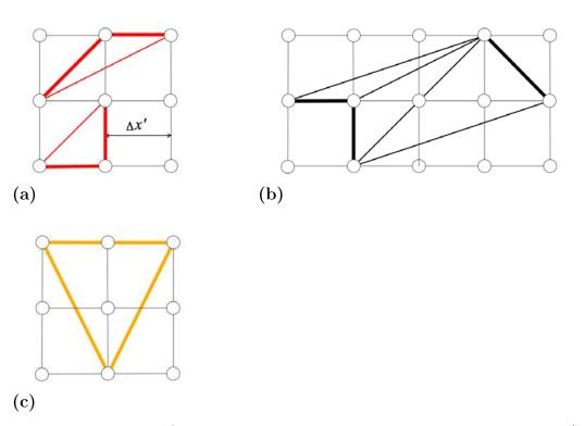
Figure 1.5: Possible facets in the convex hull projected on a regular grid (bold lines correspond to  $d_i \leq \sqrt{2} \Delta x'$ ). (a) facets in a one-phase field; (b) facets in a two-phase field; (c) three-phase field facet.
