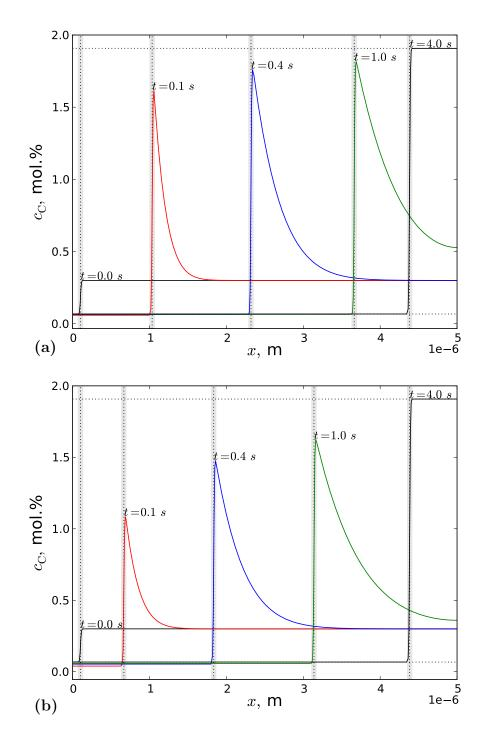
Figure E.1: Carbon concentration profiles: (a)  $M = 10^{-11} \text{ m}^4/\text{J/s}$ ; (b)  $M = 10^{-12} \text{ m}^4/\text{J/s}$ .
