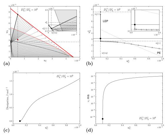
Figure 2.16: Results of the *u*-model (abscissae are  $u_{\rm C}^{\alpha}$ ) for  $D_{\rm X}^{\gamma*}/D_{\rm X}^{\gamma} = 10^6$ : (a) tie-lines; (b) nominal concentration  $u_{\rm X}^0$ ; (c) total dissipation; (d) growth rate.
