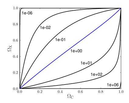
Figure 2.6: Supersaturation in X vs. supersaturation in C for various  $D_{\rm X}^{\gamma}/D_{\rm C}^{\gamma}$  ratios for a planar ferrite precipitate.
