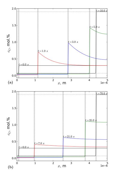
Figure E.2: Carbon concentration profiles: (a)  $M = 10^{-13} \text{ m}^4/\text{J/s}$ ; (b)  $M = 10^{-14} \text{ m}^4/\text{J/s}$ .
