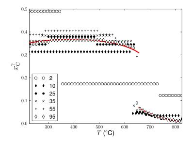
Figure 1.15: Approximate equilibrium  $x_{\rm C}^{\gamma}$  vs. temperature obtained with Quickull for Fe-0.92 mol.%C-2.66 mol.%Cr with different discretizations N (red line obtained with Thermo-Calc tcs).
