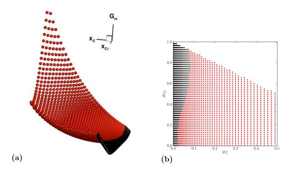
Figure 1.2: Discretized Calphad Gibbs energies of  $\alpha$  and  $\gamma$  in Fe-C-Cr using *FEDAT* database, at 600 °C (concentration axes are  $x_{\rm C}$  and  $x_{\rm Cr}$ ). Red dots are for  $\gamma$  and black ones for  $\alpha$ . Only lower dots have been plotted for clarity.
