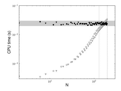
Figure 1.9: CPU times vs. N of QH (white) and subsequent NR (black) for Fe-0.5mol.%C at 600°C (triangles) and 800°C (dots).
