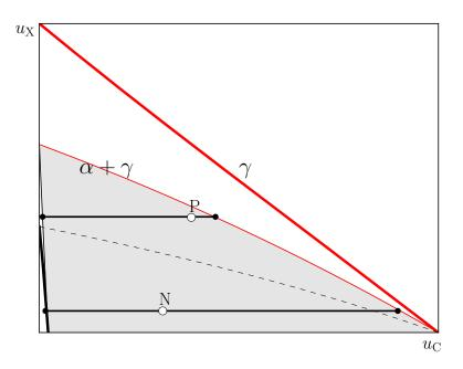
Figure 2.9: Isothermal section of a schematic Fe-C-X phase diagram with solubility limits of  $\alpha$  (thick black) and of  $\gamma$  (red). Paraequilibrium two-phase field in grey with paraequilibrium tie-lines for alloys N and P.
