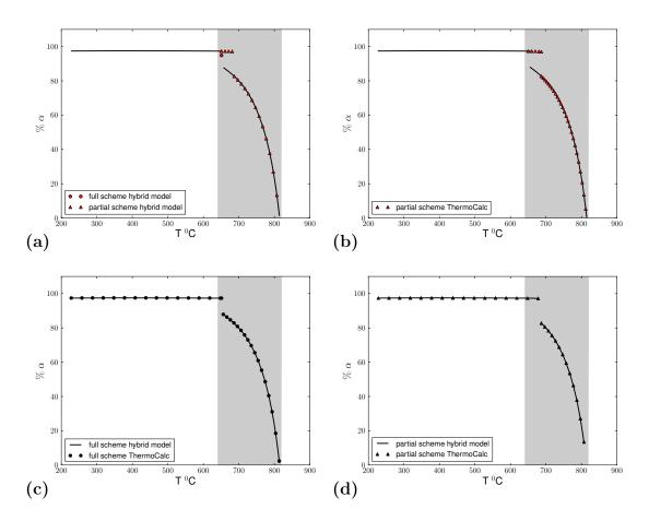
Figure 1.17: Phase fraction of  $\alpha$  vs. temperature in a Fe-0.92 C-2.66 Cr (mol.%) alloy, full scheme (dots) partial scheme (triangles): hybrid model (**a**), Thermo-Calc (**b**), hybrid and Thermo-Calc full scheme (**c**), hybrid and Thermo-Calc partial scheme (**d**).
