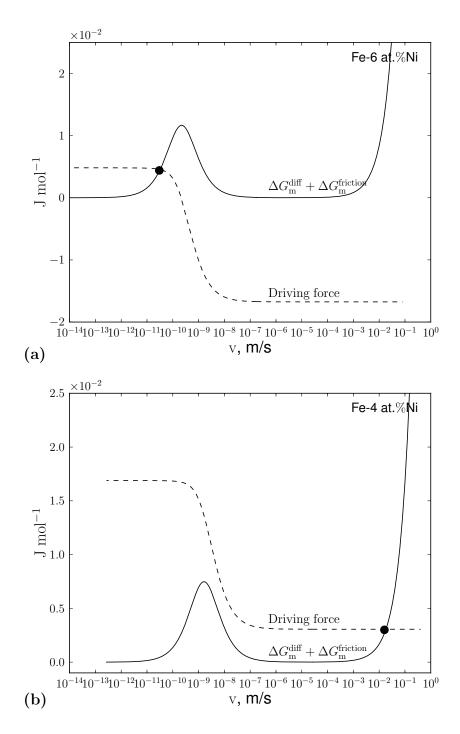
Figure 2.4: Dissipation of Gibbs energy (continuous line) and driving force (dashed line) in (a) Fe-6 at.%Ni and (b) Fe-4 at.%Ni at 727°C.
