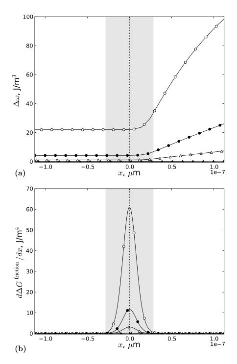
Figure 3.11: Profiles of (a) driving force  $\Delta w$  and (b) dissipation by friction  $h'(\phi)\Delta w$  at the interface (grey slab) at  $10^{-2}$  s (white dots), 1 s (black dots), 1.5 s (white triangles) and 2 s (black triangles).
