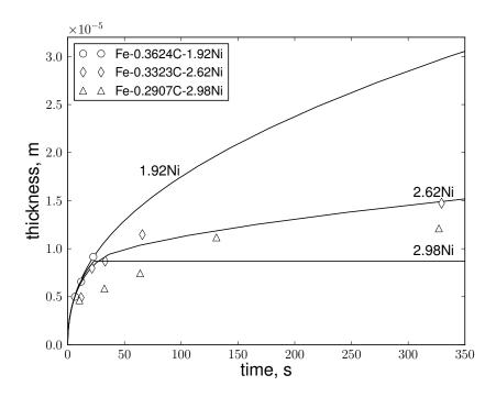
Figure 2.31: Ferrite growth kinetics in different Fe-C-Ni alloys (at.%) at 700°C (Tab. 2.2): present work (black lines) and experiments from [87] (symbols).
