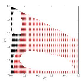
Figure 1.3: Remaining labelled nodes (black= $\alpha$ , red= $\gamma$ ) of the initial grids when non-convex parts are discarded.
