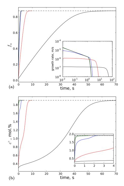
Figure 3.13: (a) Ferrite fraction and (b) interface concentration in  $\gamma$  vs. time in Fe-0.3C (wt.%) at 776°C, for different M (in m<sup>4</sup>/J/s): 10<sup>-2</sup>, 10<sup>-11</sup>, 10<sup>-12</sup>, 10<sup>-13</sup>, 10<sup>-14</sup> (from fastest to slowest).
