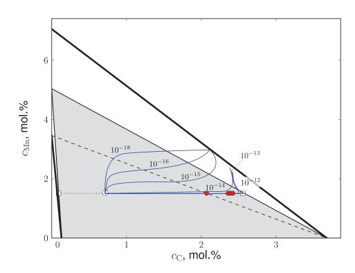
Figure 3.16: Evolutions of  $c^{\gamma}$  (blue curves) in the isothermal section of the Fe-C-Mn diagram at 650 °C for different mobilities M (in m<sup>4</sup>/J/s).
