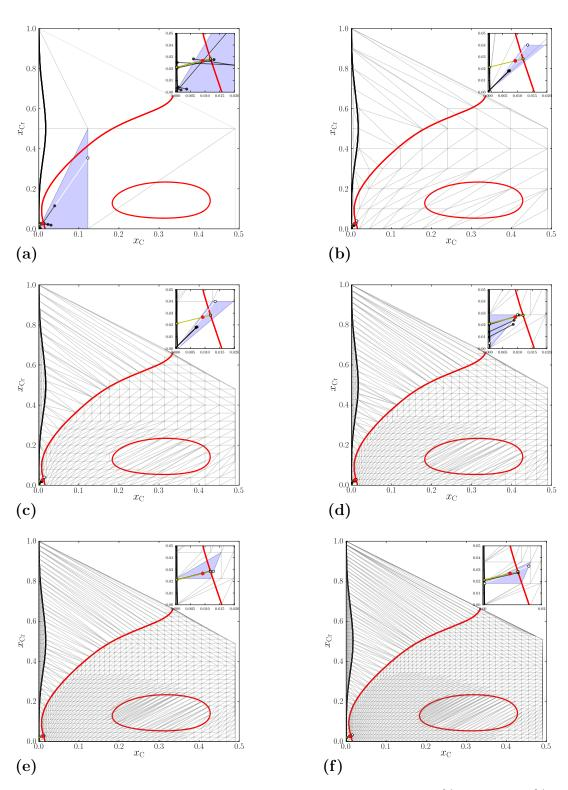
Figure 1.14: Tie-line search process with NR for Fe-0.92 mol.%C-2.66 mol.%Cr (red dot), starting with the tie-lines obtained from the convex hulls at 800°C (white line in the blue triangle) for N = 2 (a), N = 10 (b), N = 25 (c), N = 35 (d), N = 45 (e), N = 55 (f). Intermediate, and final tie-lines are in black and yellow respectively.
