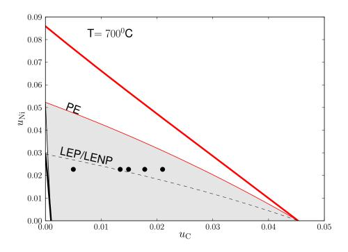
Figure 2.22: Isothermal section of the Fe-C-Ni ternary phase diagram at 700°C with the investigated alloys (black dots) in Tab. 2.1.
