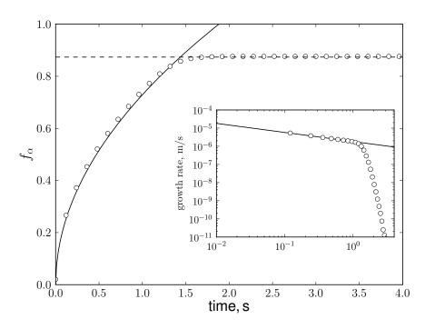
Figure 3.7: Ferrite fraction vs. time in Fe-0.3C (wt.%) at 776°C: phase field (white dots), sharp interface (continuous line) and equilibrium (dashed line).
