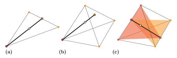
Figure 1.6: Geometrical construction for determining the approximate tie-line corresponding to the white dot: (a) ternary alloy; (b-c) quaternary alloy.
