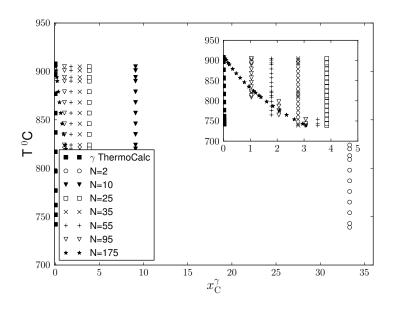
Figure 1.7: Approximate equilibrium  $x_{\rm C}^{\gamma}$  vs. temperature in Fe-C obtained with Quickhull with different discretizations N.
