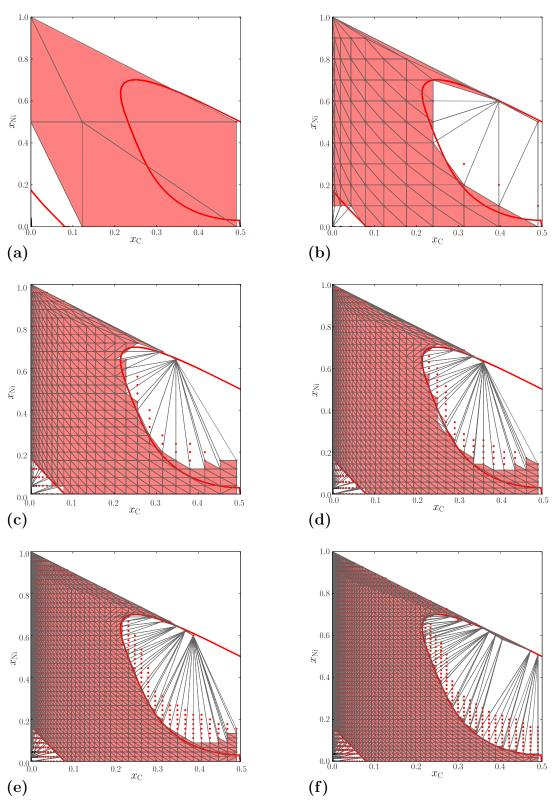
Figure C.1: Projections of the final convex hulls (triangles) of the Gibbs energies of  $\alpha$  (black dots) and  $\gamma$  (red dots) in Fe-C-Ni at 600°C, for N = 2 (a), N = 10 (b), N = 25 (c), N = 35 (d), N = 45 (e) and N = 55 (f).
