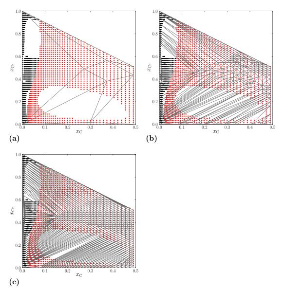
Figure 1.4: Construction of the convex hull: (a) step 10; (b) step 200; (c) final step. Triangles are the projections of the facets.
