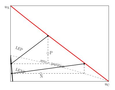
Figure 2.7: Isothermal section of a schematic Fe-C-X phase diagram with solubility limits of  $\alpha$  (thick black) and of  $\gamma$  (red). Tie-lines (thin black) with IC contours (dashed), and zero-partition line (dashed).
