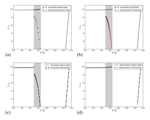
Figure 1.20: Phase fraction of  $\alpha$  vs. temperature in a Fe-0.92 C-2.66 Cr -0.81 Mo (mol.%) alloy, full scheme (dots) partial scheme (triangles): hybrid model (a), Thermo-Calc (b), hybrid and Thermo-Calc full scheme (c), hybrid and Thermo-Calc partial scheme (d).
