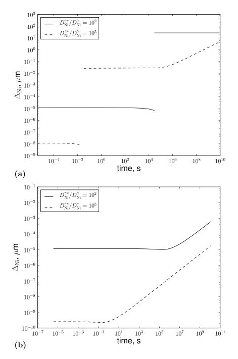
Figure 2.32: Evolution of the Ni spike width in  $\gamma$  at 700°C in (a) Fe-0.29C-2.98Ni (mol.%) above zero-partition and in (b) Fe-0.36C-1.92Ni (mol.%) below zero-partition, assuming PE as the initial condition.
