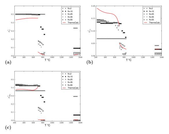
Figure 1.18: Equilibrium  $x_{\rm C}^{\gamma}$  (a),  $x_{\rm Cr}^{\gamma}$  (b),  $x_{\rm Mo}^{\gamma}$  (c)vs. temperature estimated with Quickhull for Fe-0.92 mol%C-2.66 mol.%Cr-0.81 mol.%Mo with different discretizations N and with Thermo-Calc (red line).
