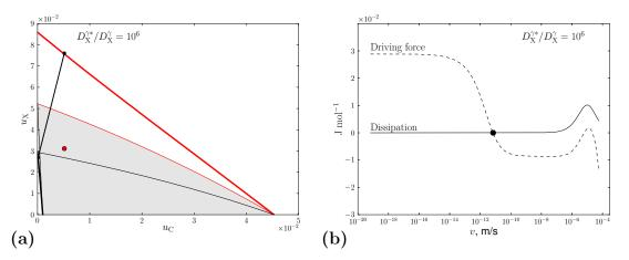
Figure 2.19: Results of the v-model (abscissae are v) for  $D_{\rm X}^{\gamma*}/D_{\rm X}^{\gamma} = 10^6$ : (a) tielines; (b) Dissipation and driving force.
