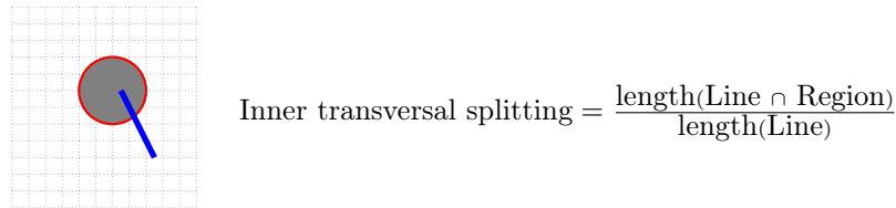
Figure 2.8: Inner transversal splitting example based on [Egenhofer and Shariff, 1998].
