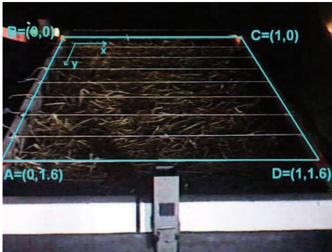
Figure A1. Schematic view and dimensions of the study area (propagation zone).
