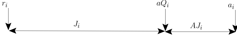
Figure 3.7: The time line of message \mu_i from its initiating event until it is able to participate in bus arbitration.
