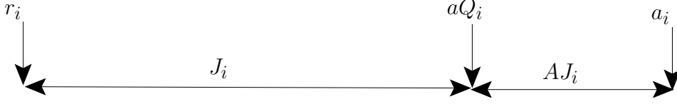
Figure 3.7: The time line of message \mu_i from its initiating event until it is able to participate in bus arbitration.
