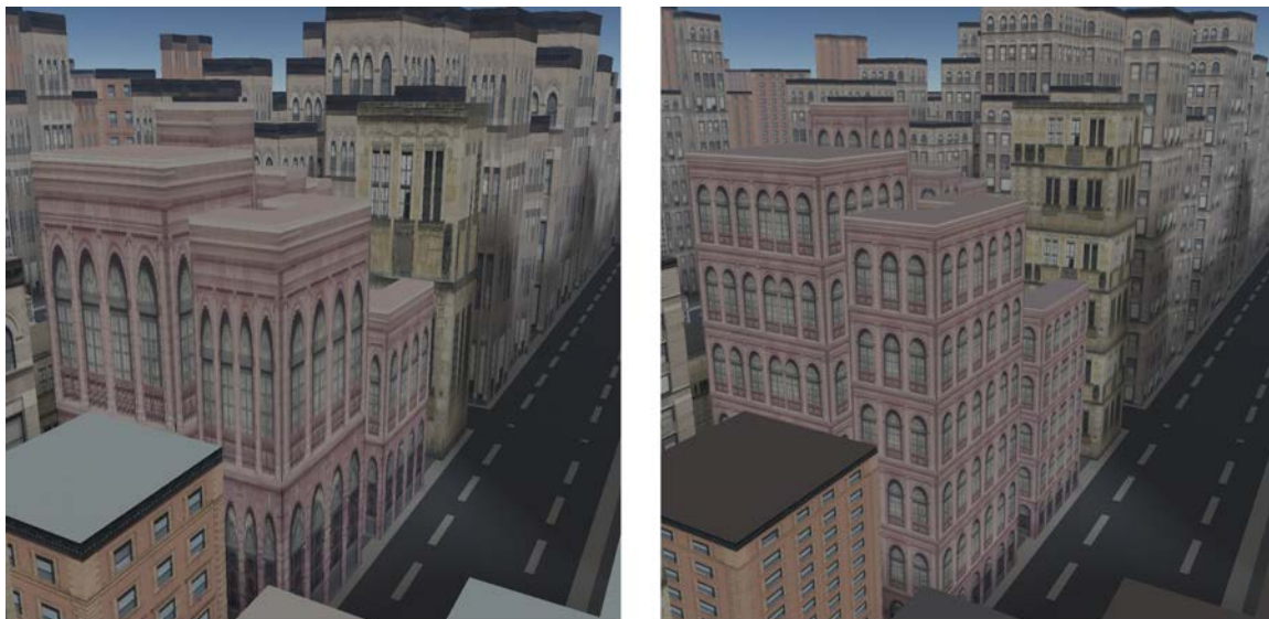
Figure 5.14: Left: The exemplars are simply stretched to fit the facades. Right: The synthesizer adapts the exemplars to best fit the facades. This greatly improves quality but rendering is more than 3 times slower.
