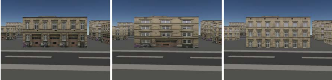
Figure 5.1: Three different methods used to adapt textures to their supporting surfaces Left: Texture synthesis. Middle: Stretching. Right: Tiling and cropping.
