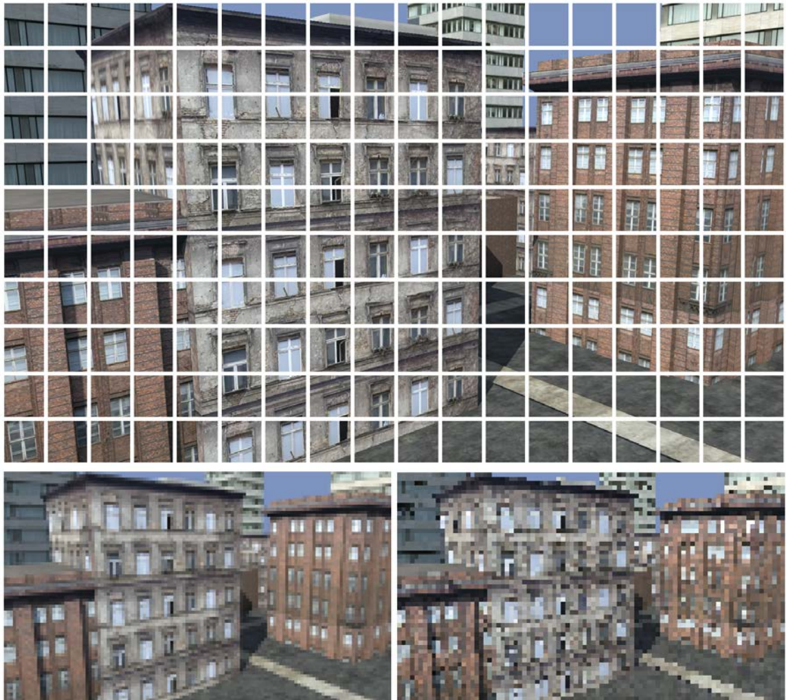
Figure 2.3: Top: Many texels are project in each pixel of the screen frame buffer. This frame buffer has a size of 18 \times 10 pixels where each pixel is represented with small squares. Bottom-left: All texels in each pixel are averaged to produce a final filtered result. Bottom-right: Among all texels projected in each pixel, a single one is selected and this produces aliasing artifacts.
