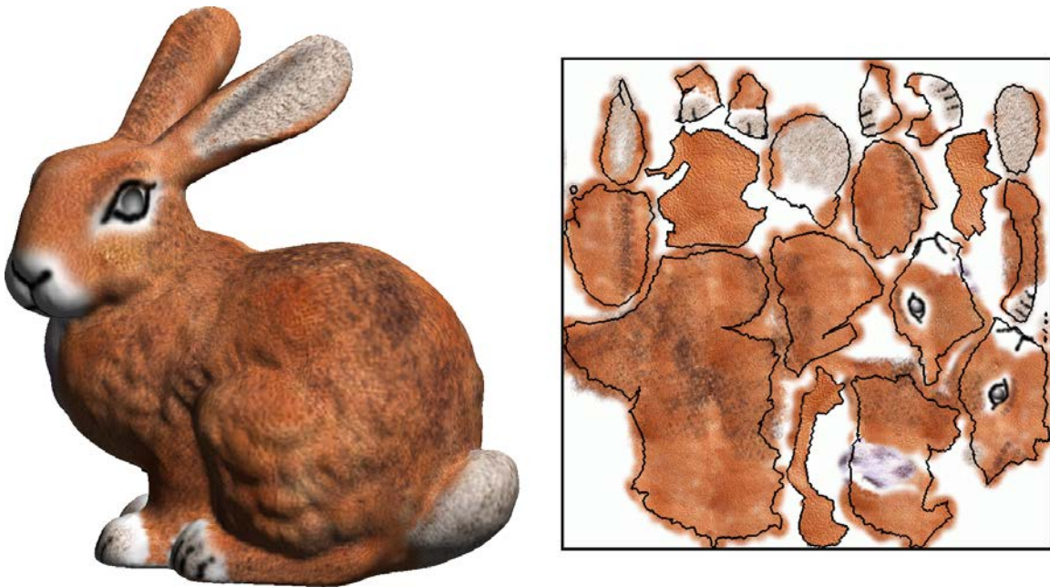
Figure 2.7: Left: Textured Stanford bunny model. Right: Texture Atlas. Source: Lévy et al. [LPRM02].
