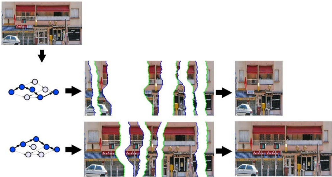
Figure 5.6: The algorithm synthesizes textures by reordering strips of the exemplar. Each result is a path in a graph describing the space of synthesizable textures.
