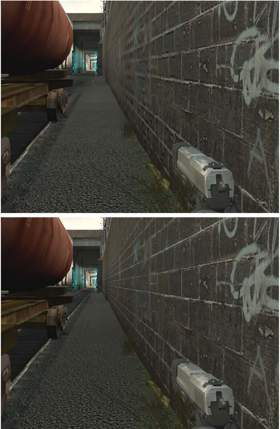
Figure 2.6: Top : Isotropic filtering. Bottom : Anisotropic filtering. Notice how the bricks on the wall, the ground and the train railroad are better preserved in the bottom image. Source : Half-Life 2 , Valve Corporation.
